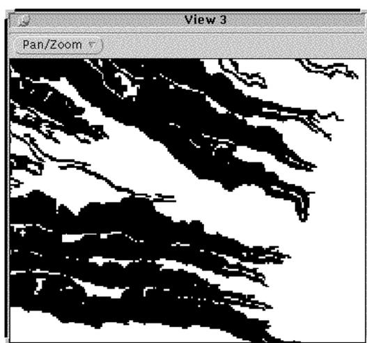
Figure 3: DEM window showing valleys after a 12 degrees threshold
