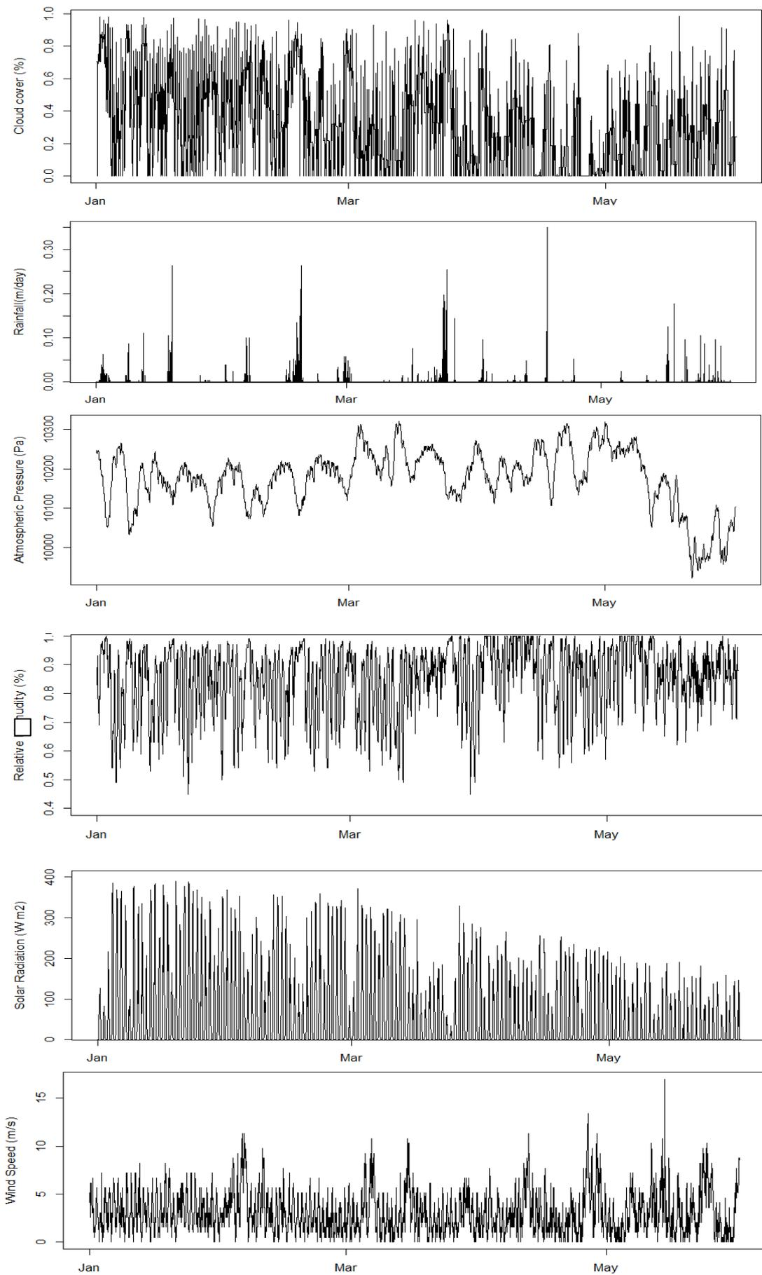
**Figure 16: Meteorological data used as input into the ELCOM model (01/01/2016 to 01/06/ 2016). From top: Cloud cover, rainfall, Atmospheric Pressure, Relative Humidity, Solar radiation and wind speed.**
