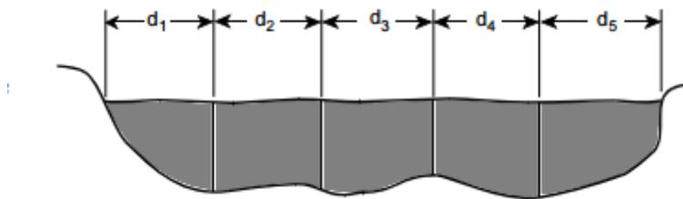
**Figure 10: Cross -section of stream verticals along the width of a stream (image FLO-MATE manual, Marsh McBriney 1990), verticals were spaced 10 cm apart due to size of waterways.**
