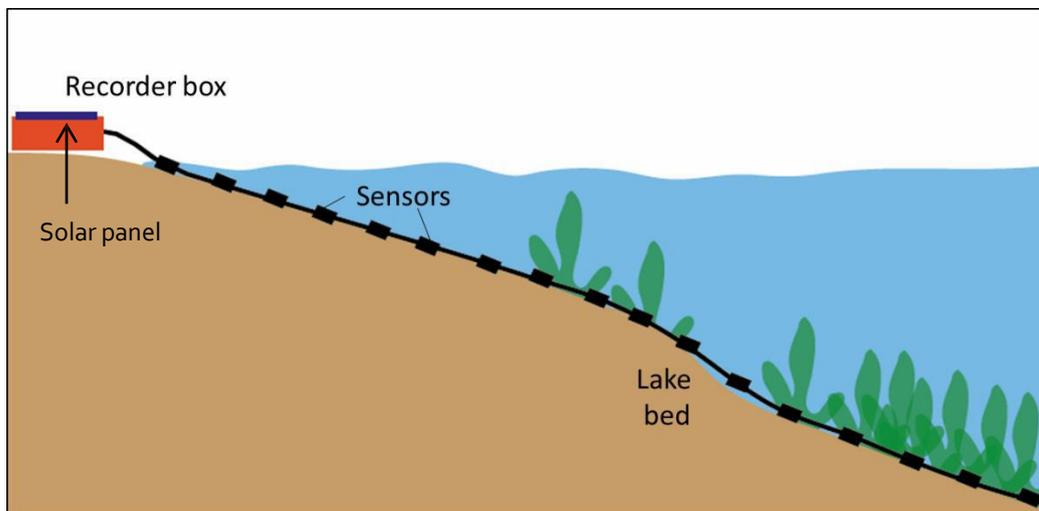
**Figure 11: Diagram showing how thermistor chain was placed on lake bed. Each sensor was 1 meter apart and a total of 20 sensors were on the chain which was connected to power box with a solar panel.**
