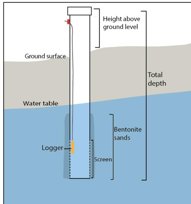
**Figure 9: Diagram showing piezometer components and installation.**
