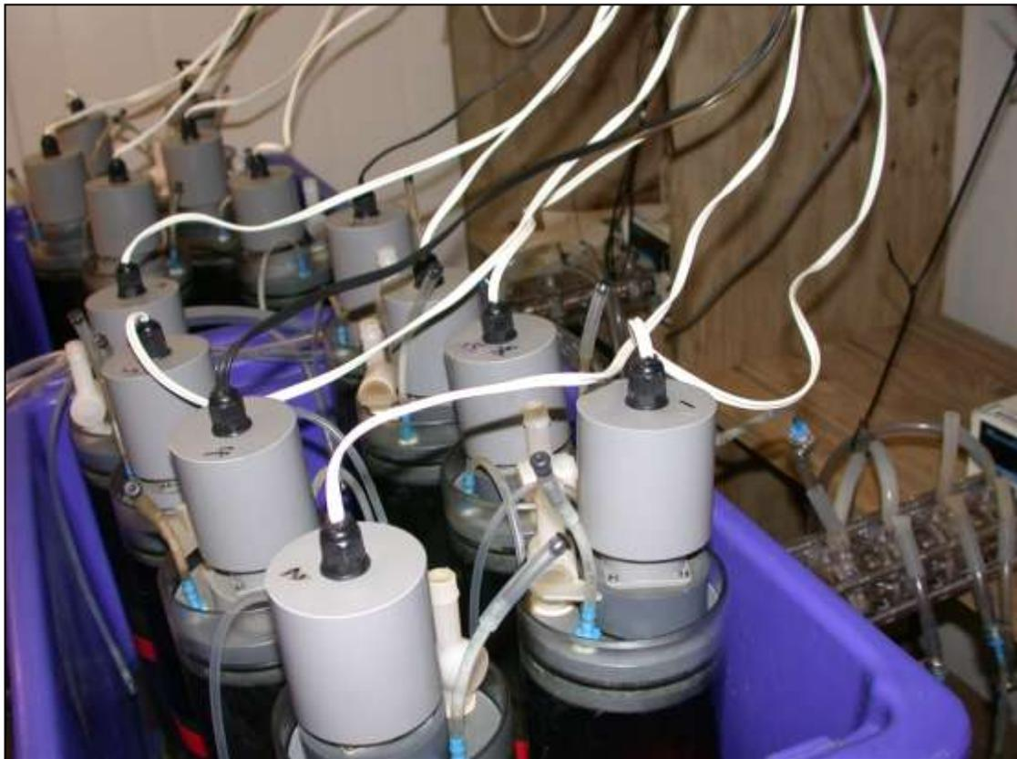
Figure 12. Core incubation set-up with peristaltic pumps visible to the right of the blue basins. The sealed ends of the tubes used to cycle lake water through the cores are clearly visible in the foreground. White taps were used to place the oxygen sensor into the water column and withdraw water samples for nutrient analysis. The cylinders on top of the cores are the magnetic stirrers used to prevent stratification during the experiment.
