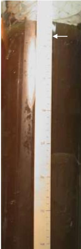
Figure 9 Photo of the top of one of the settling columns used in the experiment. The white arrow indicates the location of the sediment-water interface. This photo was taken after 117 h of settling in the  $90 \text{ g L}^{-1}$  sediment concentration, showing a depth of approximately 38 mm.
