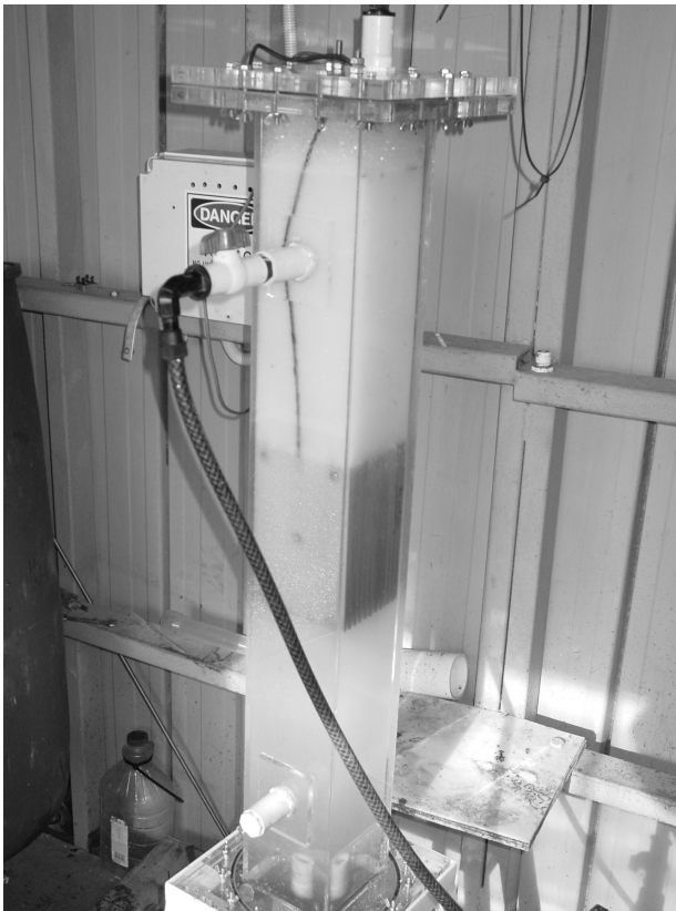
Figure 3-15 Down-flow electroflotation clarifier. Algae and other particulates were raised above the inflow point in sturdy foam. Some small bubbles passed down beyond the processor to the outflow stream at the bottom. Some of these small bubbles coalesced to form larger bubbles that rose back up through the processor.
