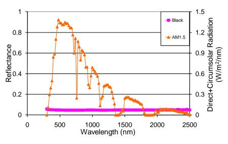
Fig. 4 Reflectance from black steel sample over AM1.5 spectrum
