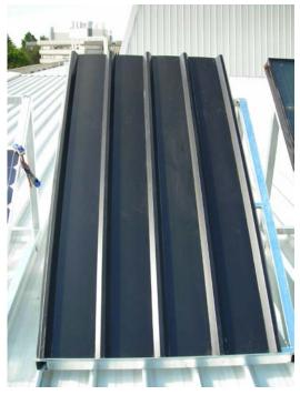
Fig. 3 Prototype building integrated solar collector
