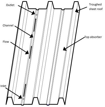
Fig. 2 Building integrated solar collector
