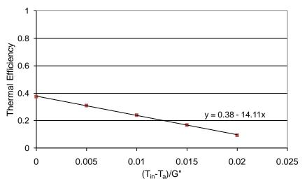
Fig. 5 Theoretical efficiency of unglazed black collector
