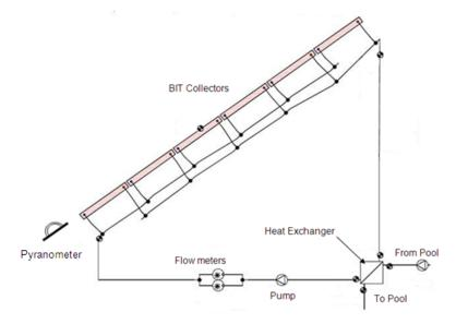
Fig. 7 Schematic of Dive Pool System
