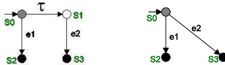
Figure 3.14: Automaton  $A_2$  (right) shows automaton  $A_1$  (left) after applying the Removal of  $\tau$ -Transitions Leading to Non- $\alpha$  States rule.
