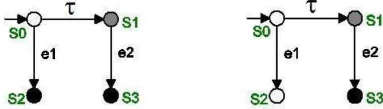
Figure 3.9: Automaton  $A_2$  (right) shows automaton  $A_1$  (left) after applying the removal of  $\omega$ -markings rule.
