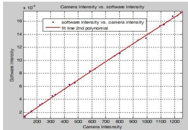
Figure 7: 2<sup>nd</sup> degree poly-fit of intensity function.
