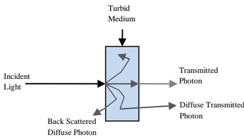
Figure 1: Light scattering and absorption in turbid medium.
