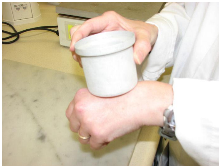
Figure 22: Measuring 'Room Temperature' using the back of a hand. A recorded temperature that is too "Hot" or too "Cold" will affect the test result.
