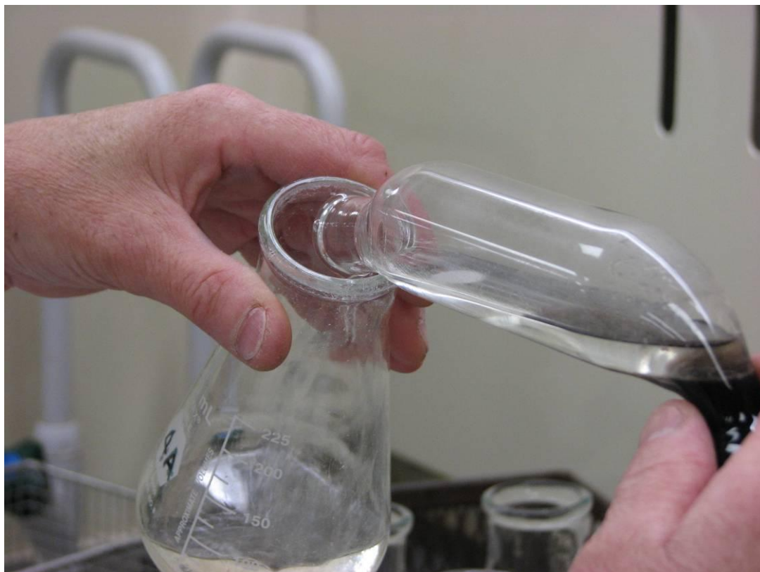
Figure 23: Decanting from a Mojonnier Flask – the skill of the technician lies in knowing how to pour off the surplus liquid accurately, leaving just the dark coloured layer behind.
