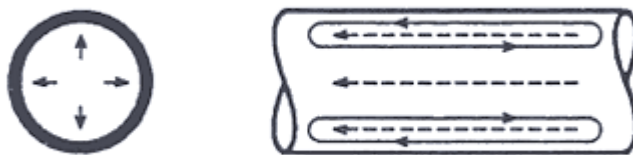
Figure 2.22: Eddy current at high frequency (Dixon Jr, 1988)
