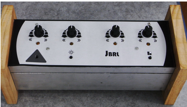
Figure 2: Mock-up of the enclosure for presentation to branding and software groups. The end-plates are arranged to present the panel tilted forward.
