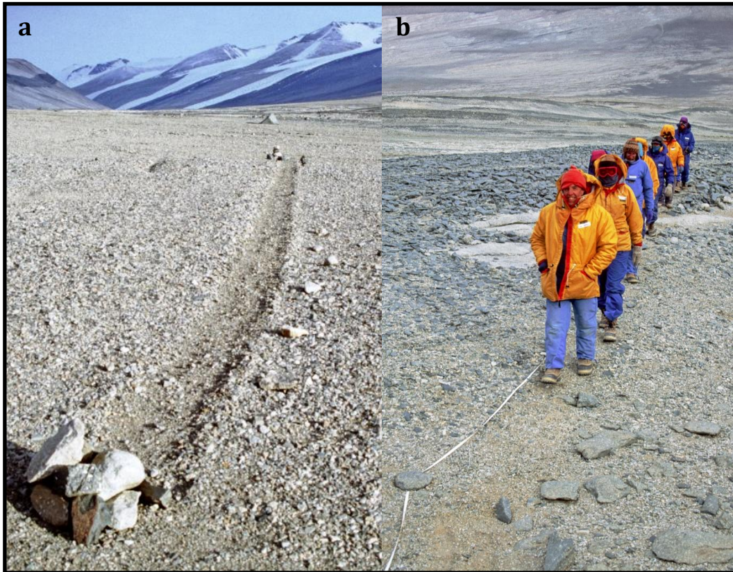
Fig. 13. Vanda Treading Trial Experiment, Wright Valley, McMurdo Dry Valleys. a) Vanda Fan site after 200 passes, 1993/94; b) Vanda Rocky site after 192 passes (last pass, 8 people), 1993/94. Photos: Megan Balks.
