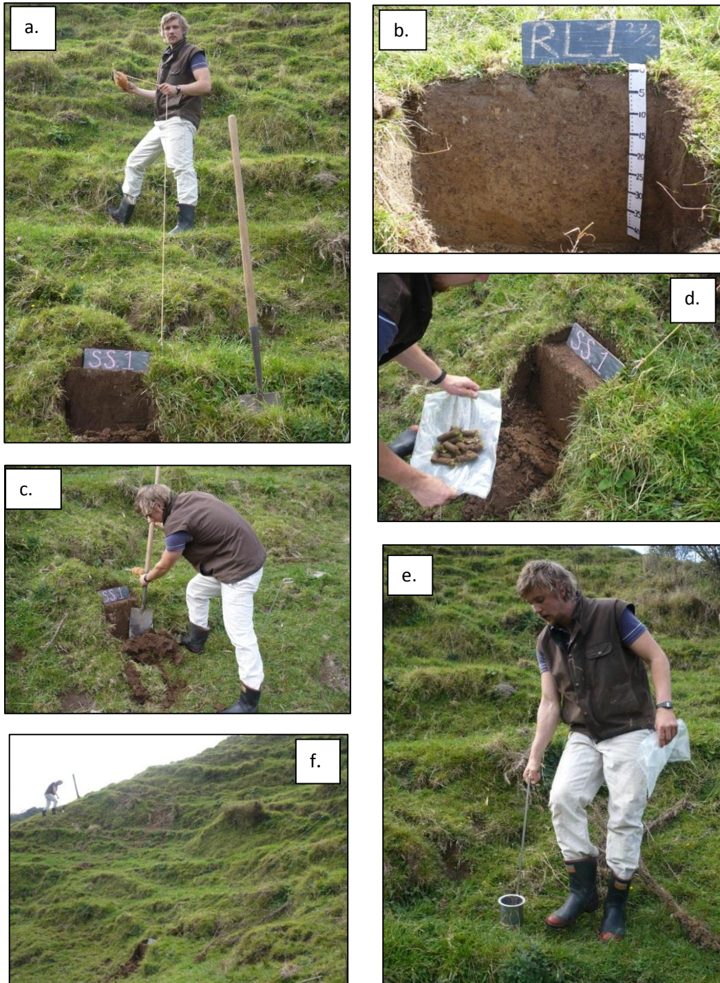
Figures 3.7 - Summary of sample process - a - Laying out 40 m transect with 2 m interval - b - Soil profile to allow for profile description - c - Digging soil pits at each end of the transect - d - Bulking the samples at the end of the transect - e - Taking samples every two metres over the 40 m transect - f - Pacing out 10 m to sample the grid
