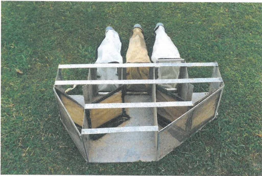
Plate 5.3 Hobbs and Butler (1981) Combination upstream migration/drift sampler, with lid removed to show internal design.
