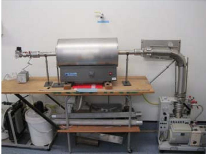
Figure 2.2: Stainless steel vacuum tube furnace.
