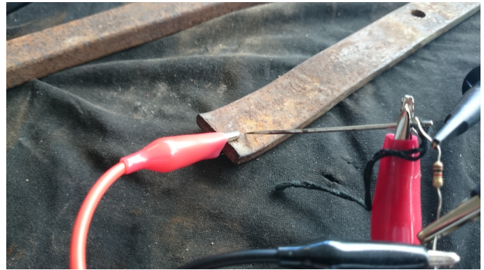
Fig. 2. Photo showing experimental setup of Rust Joint
