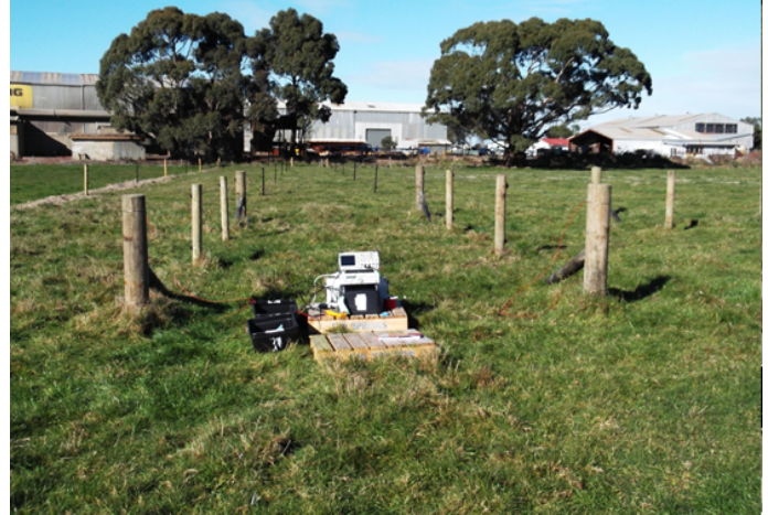
Fig. 4. The fence constructed for testing the impact of various components on the energizer communications system
