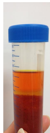
Figure 3-1: Centrifuged sample showing organic and aqueous layers
