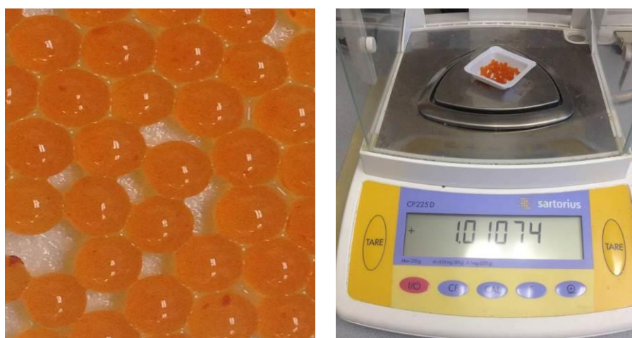
Figure 4-35: Chitosan coated lycopene alginate-agar beads
