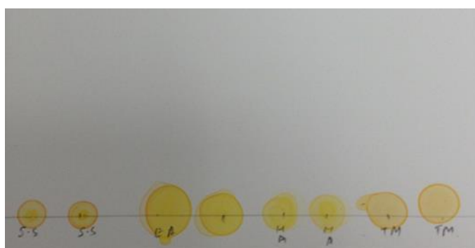
Figure 3-8: TLC silica plate with drop of lycopene extract
