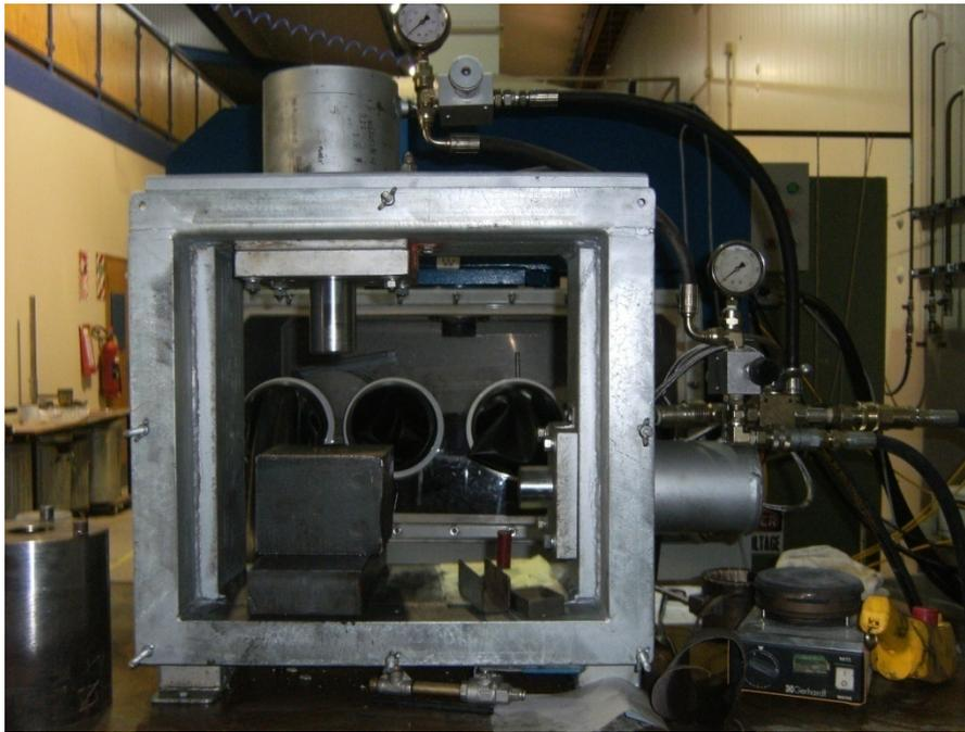
**Figure 3.3** Hydraulic press and the rigid die used for the powder/spacer material mixture.
