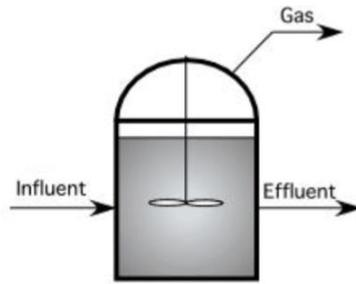
Figure 2-14: Completely stirred tank reactor (CSTR), (*Dairy Waste Handbook*, 2000).
