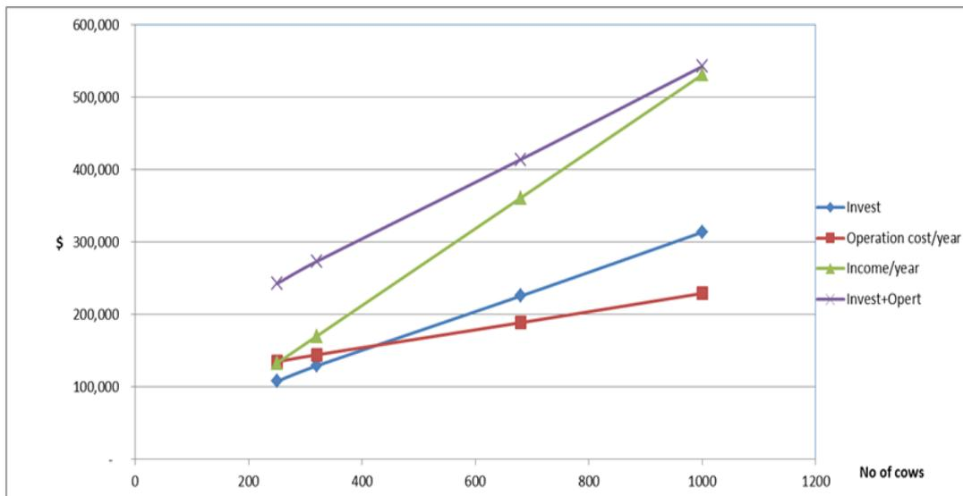
Figure 8-1: Cost analysis per herd size for anaerobic digester
