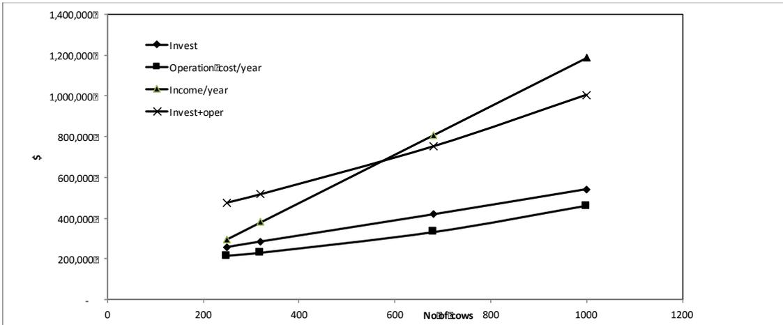
Figure 5-11: Cost analysis for three stage coupled mesophilic biodigester
