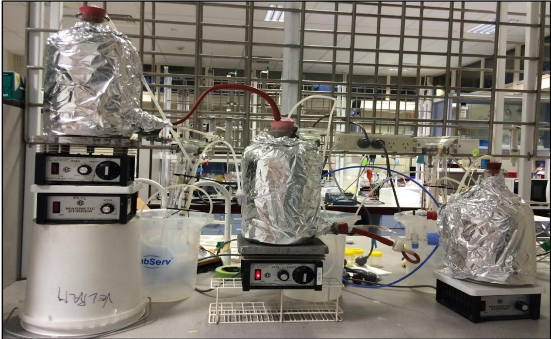
Figure 3-3: Bench scale coupled methanogenic three-stage bio-digester
