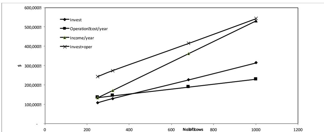
Figure 5-9: Cost analysis for anaerobic digester
