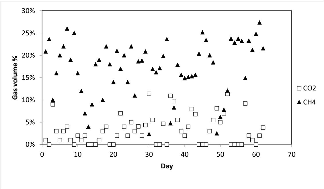
Figure 4-15: CH<sub>4</sub> and CO<sub>2</sub> gas volume percentage for reactor 7
