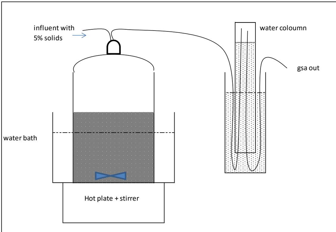
Figure 3-2: Schematic representation of the 1L benchscale reactor
