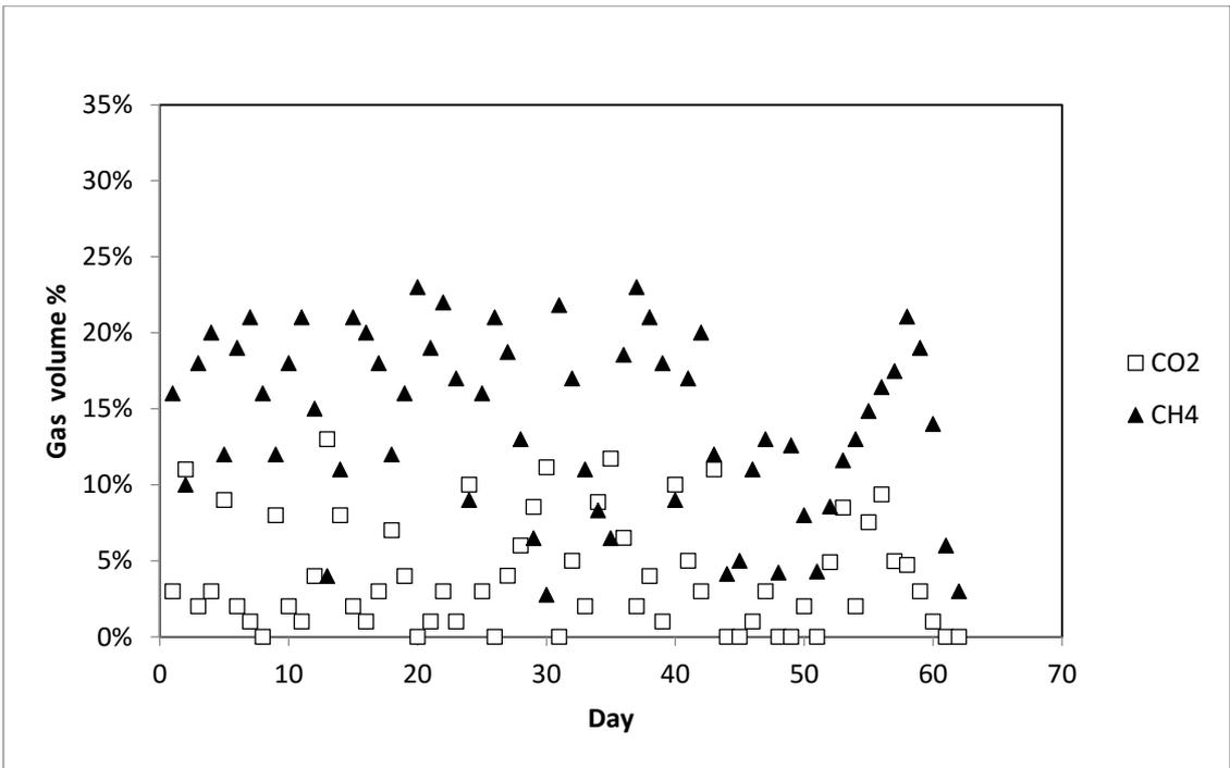
Figure 4-16: CH<sub>4</sub> and CO<sub>2</sub> gas volume percentage for reactor 8
