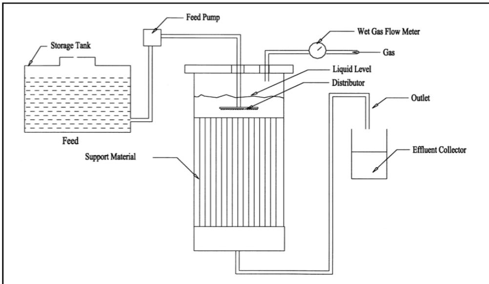
Figure 2-18: Fixed film reactor (Rajeshwari, Balakrishnan et al. 2000).
