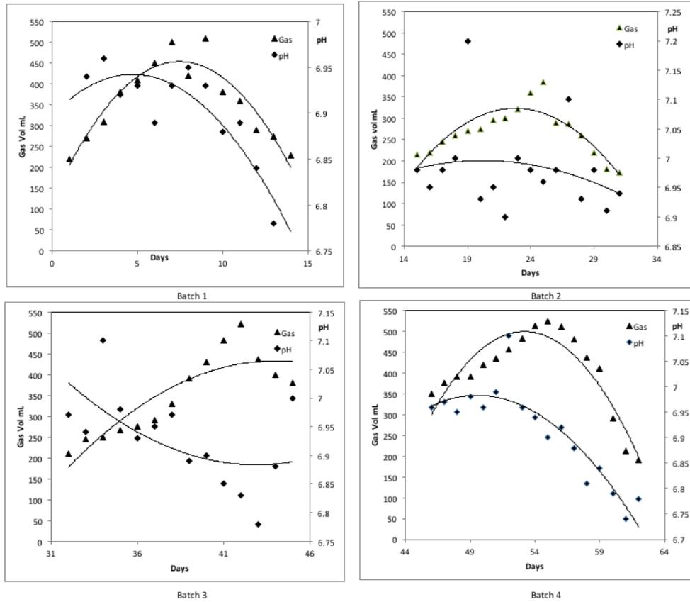
Figure 4-6: Gas volume (mL) in comparison to pH changes in Reactor 7, with batch addition of new effluent
