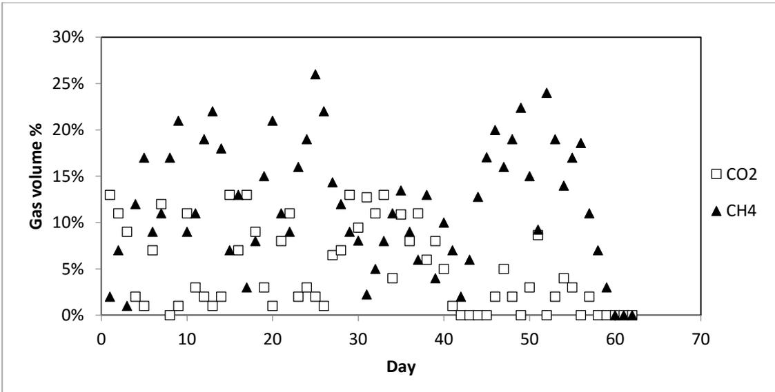
Figure 4-17: CH<sub>4</sub> and CO<sub>2</sub> gas volume percentage for reactor 9
