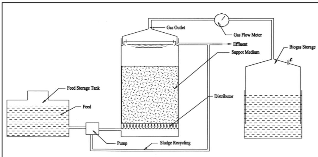
Figure 2-17: Fluidised Bed Reactor (Rajeshwari, Balakrishnan et al. 2000).
