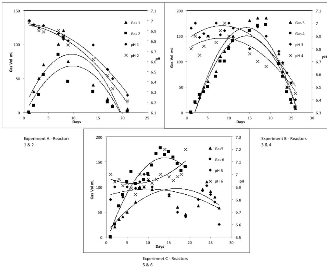
Figure 4-5: Gas volume(mL) in comparison with the pH changes in Experiments A, B and C (Reactors 1-6)
