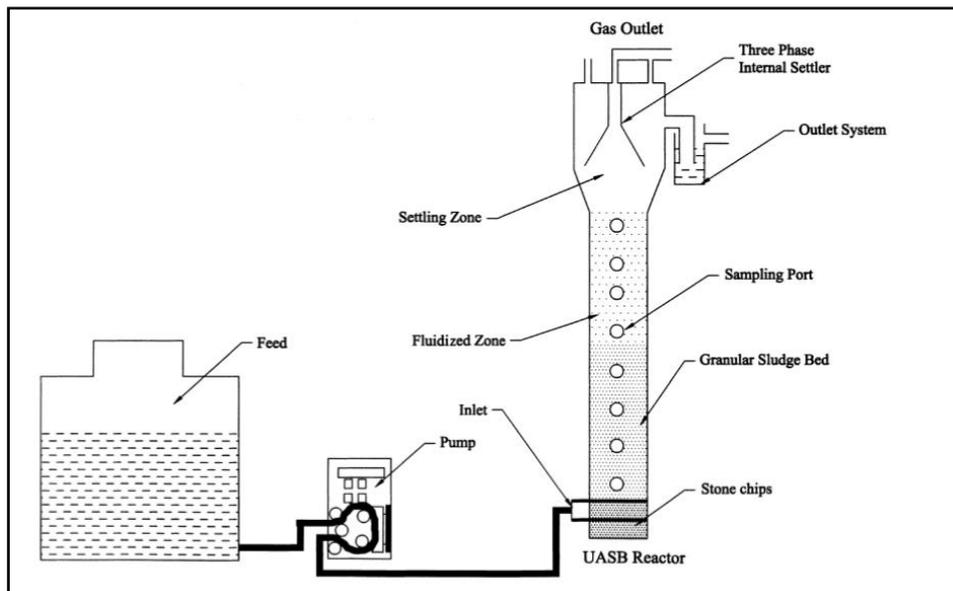
Figure 2-15: Generic UASB reactor arrangement (*Rajeshwari, Balakrishnan et al.* 2000).
