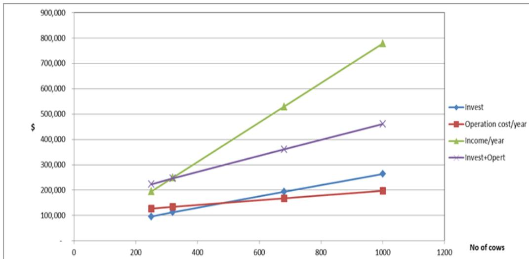
Figure 8-2: Cost analysis per herd size for plug flow digester
