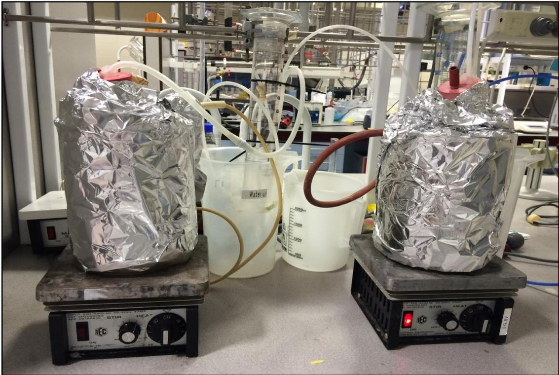
Figure 3-1: Bench scale 1L methanogenic reactor set up.
