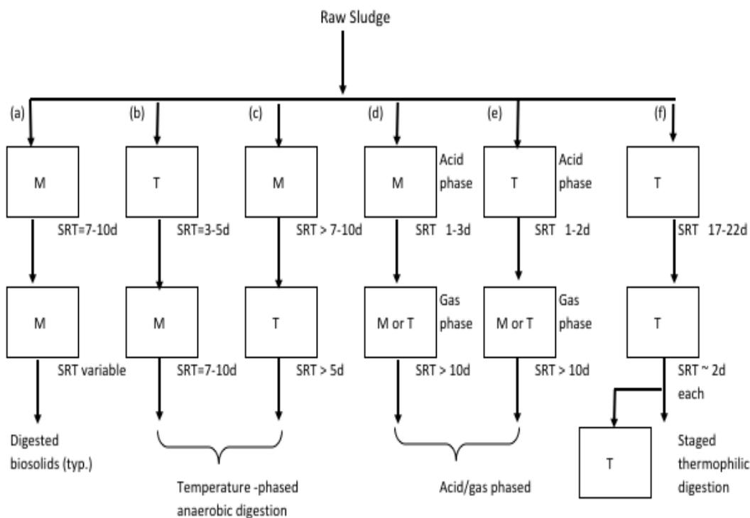
Figure 2-21: Options for staged anaerobic digestion (a) staged mesophilic digestion, (b) temperature phased thermophilic- mesophilic digestion, (c) temperature phased mesophilic-thermophilic digestion, (d) acid/gas phased digestion with mesophilic acid-phase, (e) acid/gas phased digestion with thermophilic acid phase, and (f) staged thermophilic digestion. (Adapted from Schafer and Farrellm, 2000 and Moen, 2000)
