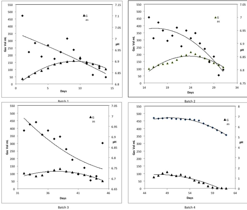
Figure 4-8: Gas volume (mL) in comparison to pH changes in Reactor 9, with batch addition of new effluent
