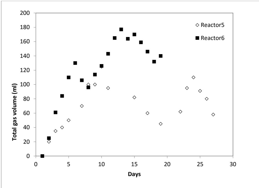
Figure 4-13: Experiment C: Reactor 5 and Reactor 6, Total gas volume (ml)
