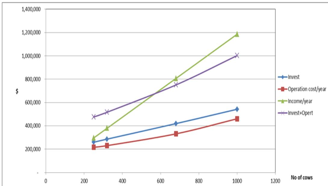
Figure 8-3: Cost analysis per herd size for three stage coupled methanogenic digester
