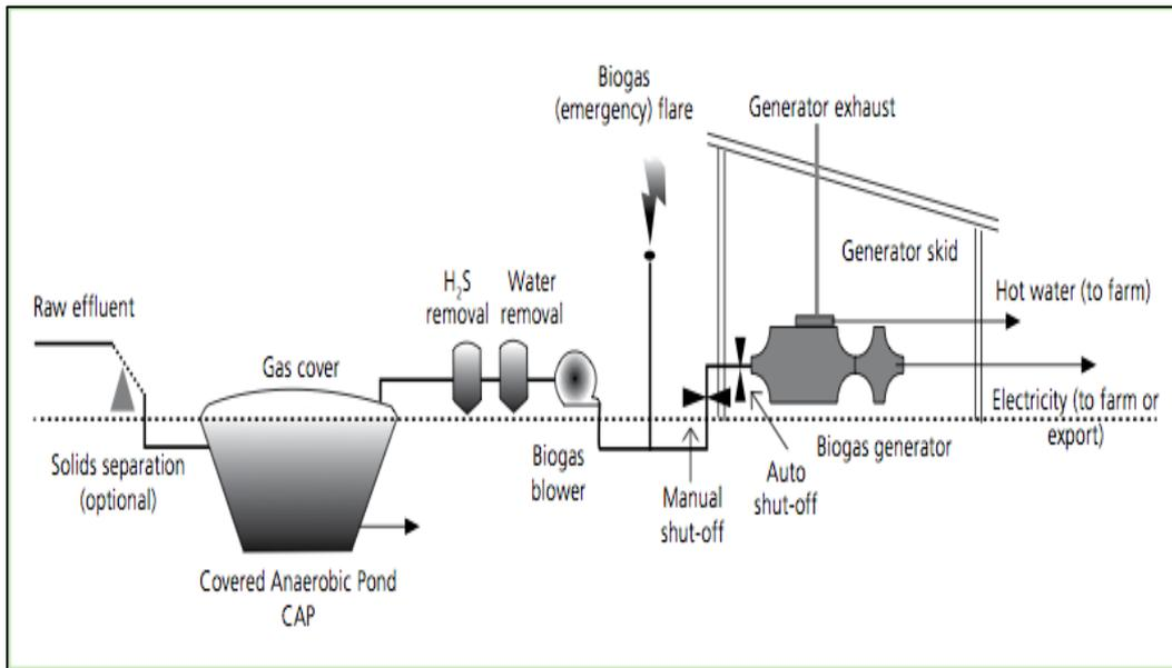
Figure 2-19: Covered anaerobic pond system (Dairy NZ, 2015)
