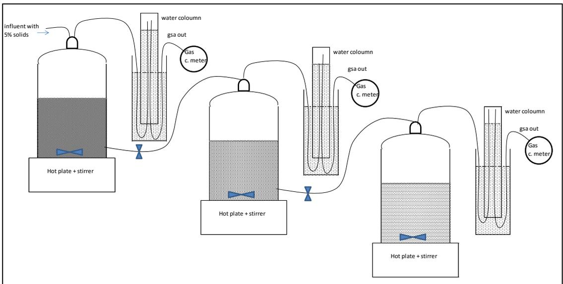
Figure 3-4: Schematic representation of continuous coupled three-stage bench-scale methanogenic reactor
