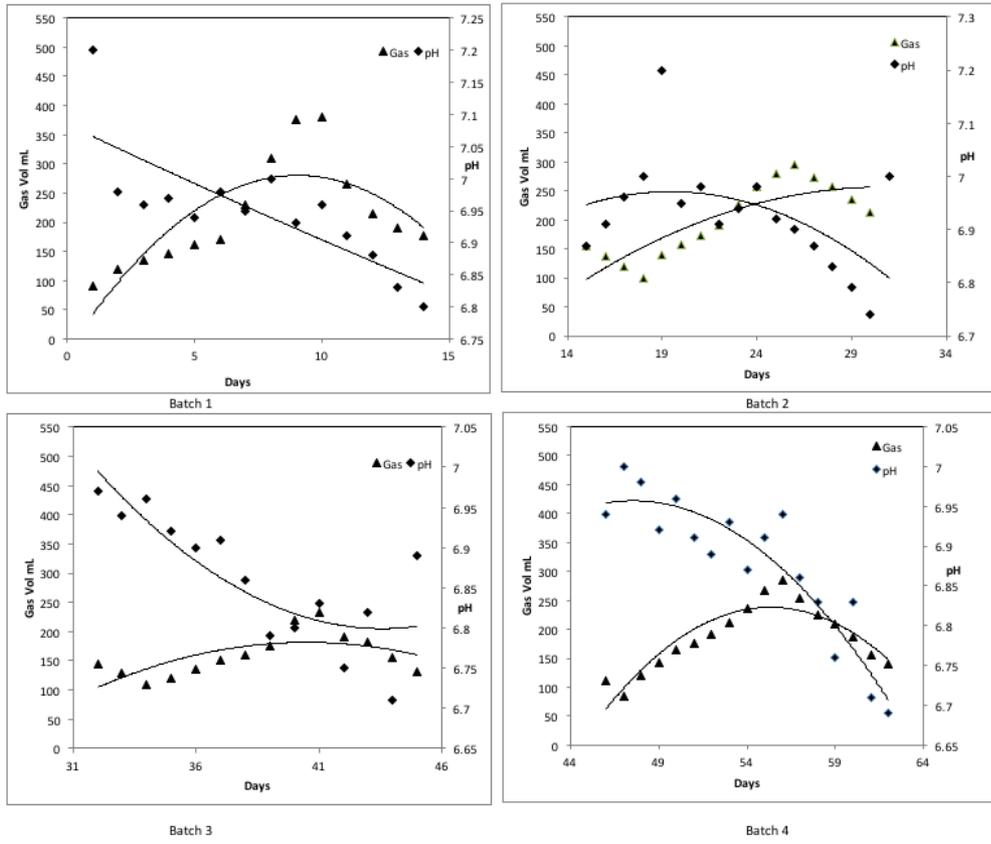
Figure 4-7: Gas volume (mL) in comparison to pH changes in Reactor 8, with batch addition of new effluent
