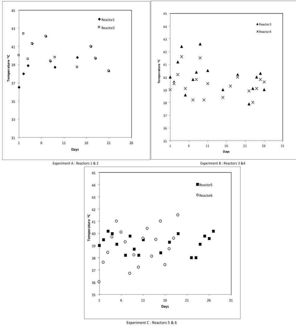
Figure 4-9: Temperature variation of Reactor 1 to 6
