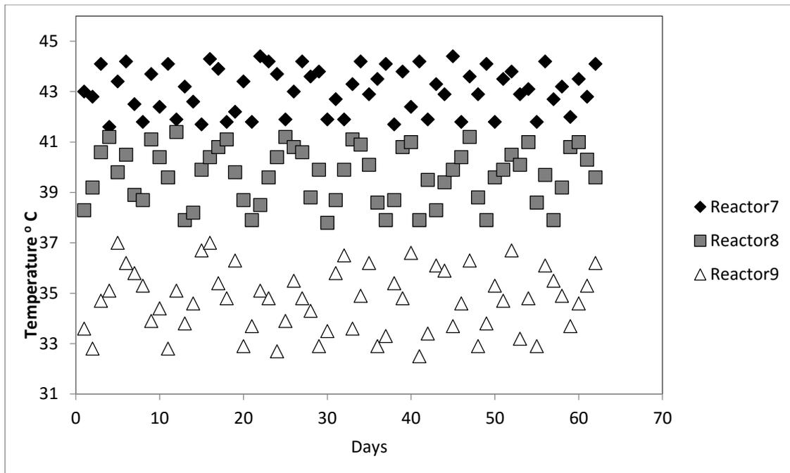
Figure 4-10: Temperature variation of Reactor 7 to Reactor 9
