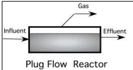
Figure 2-16: Schematic of plug flow reactor (Dairy Waste Handbook, 2000).
