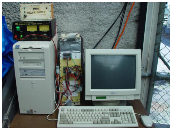
Figure 2.7. Computer equipment, including the computer components, the interface cabinet and power supplies for unit and some of the enrichments. This was housed in the indoor component of the chimpanzee enclosure, within the Keepers section.
