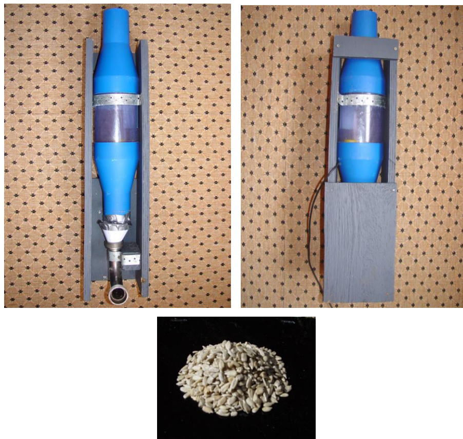
Figure 2.25. Screwfeeder, from the front (top, left) and back view (top, right), and sunflower seeds (bottom).
