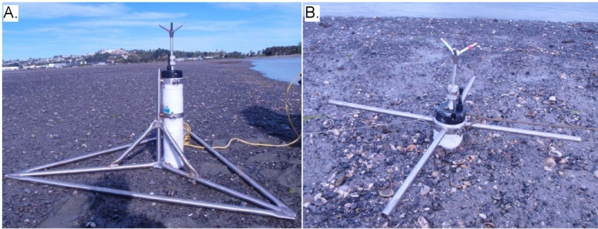
Figure 3.2. Sontek Triton-ADV current meters used in field deployment. A. Steel frame used for deployment in the channel at sites ENT and BRI. B. Steel frame used to stabilise buried instrument.
