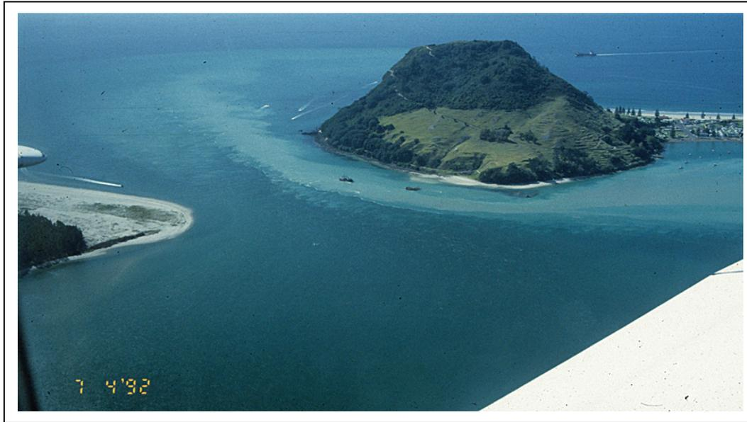
**Figure 14.** Oblique aerial view of a turbid plume generated during the 1992 capital dredging by a cutter suction dredge operating in Stella Passage.
