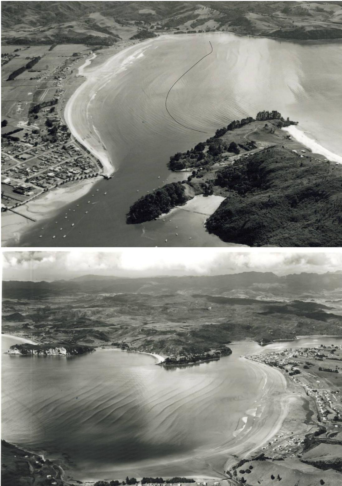
Figure 2.4 The wave refraction patterns in Buffalo Bay looking north (top) and looking south (bottom). The dotted line illustrates the curvature of the wave line along Buffalo Beach. Photos taken in 1962. Source: Environment Waikato.
