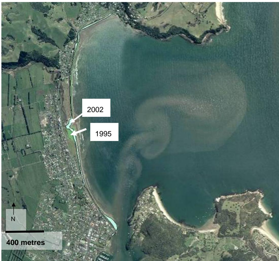
*Figure 3.7 Mercury Bay 2002 showing the large plume of sediment exiting the Whitianga Harbour. The green area shows the beach area in 1995 and the outlined area shows the beach area for 2002. Source: LINZ, 2006*
