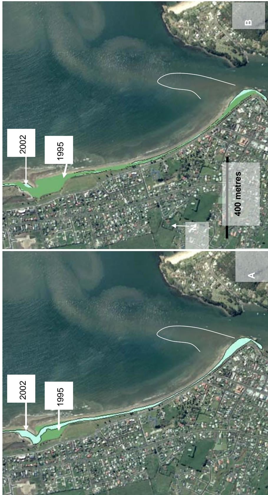
Figure 3.8 The beach area change from 1995 to 2002 for the southern section of Buffalo Beach. The dark green area shows the beach area for 1995 and the aqua area shows the beach area for 2002. Photo A has the 2002 area over top of the 1995 area, and photo B shows the 1995 area on top of the 2002 area. The white line indicates the approximate position of the ebb delta. Source: LINZ, 2005
