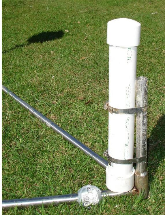
*Figure 4.4 An example of the type of sediment traps used, seen attached to the S4 frame. The cap on top of the trap is removed after they are deployed. Photo taken by author.*
