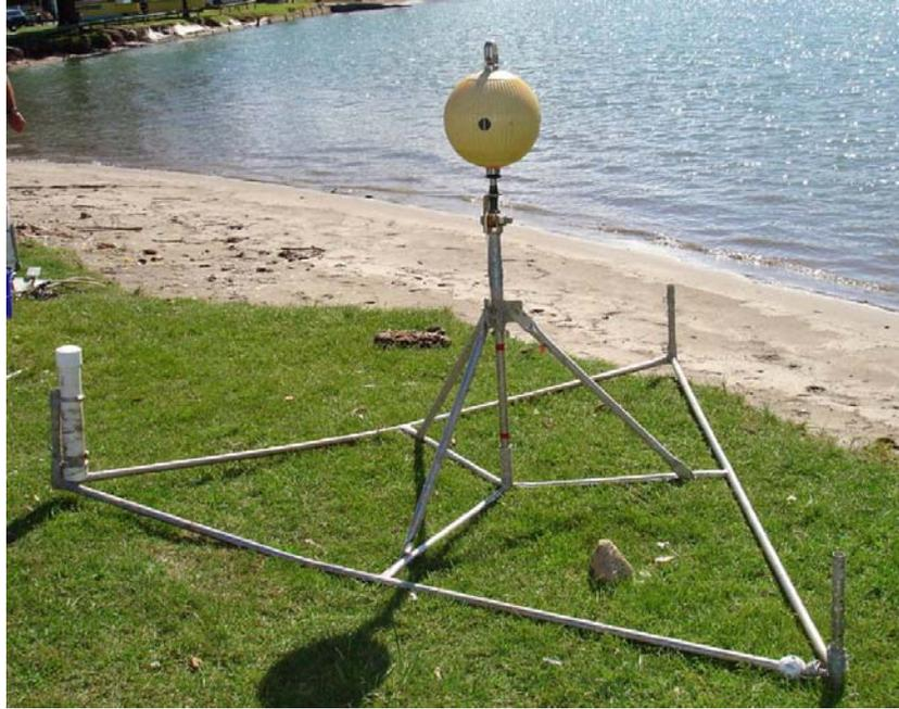
*Figure 4.2 The S4 current meter with its frame. Sediment traps were fastened to the sides, as seen to the left of the photo. Photo taken by author.*
