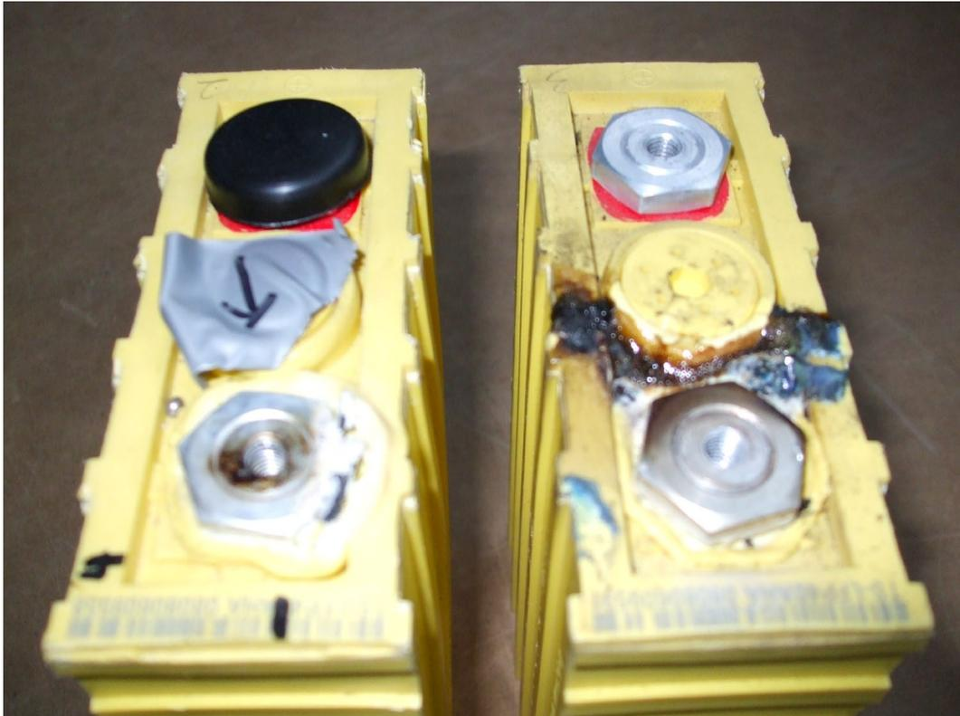
**Figure 7.20** Heat damaged battery terminals of a Li-ion cell caused by excessive discharge current under abuse conditions.
