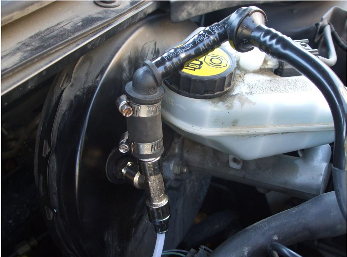
**Figure 8.6** Tee junction and pneumatic line for vacuum gauge.
