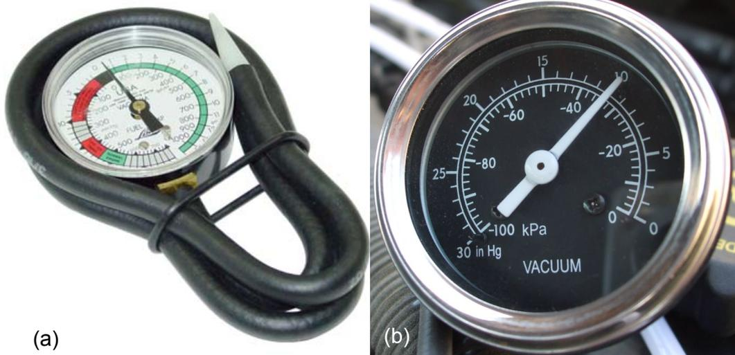
**Figure 8.5** (a) Automotive vacuum test gauge 0 to -100 kPa (anticlockwise) integrated with fuel pump pressure tester (b) Vacuum gauge 0 to -30 inHg (100 kPa) (anticlockwise).
