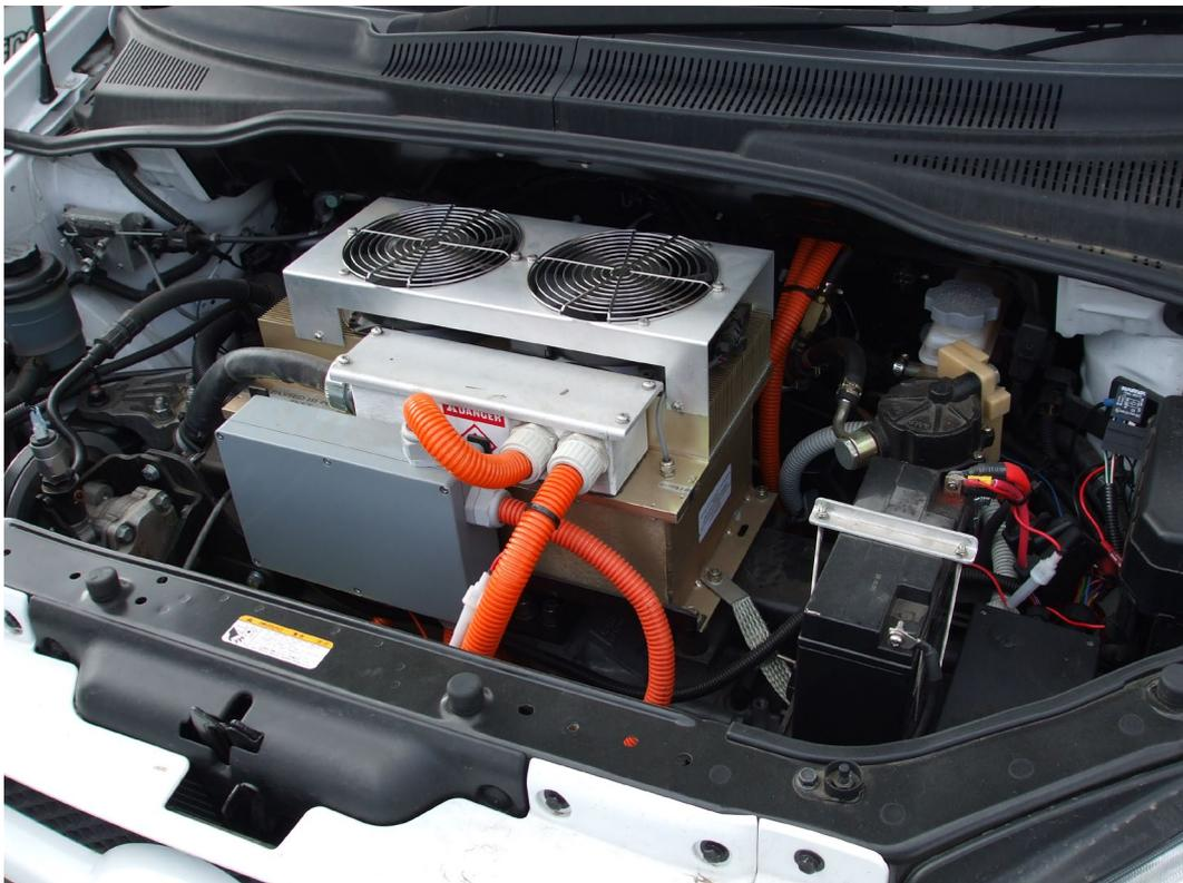
**Figure 6.7** Blade Electron professional EV conversion.
