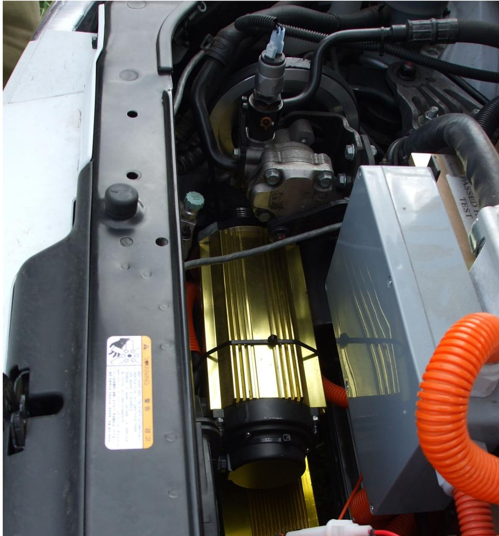
**Figure 9.1** The power steering motor (retrofitted) and pump in an EV conversion.
