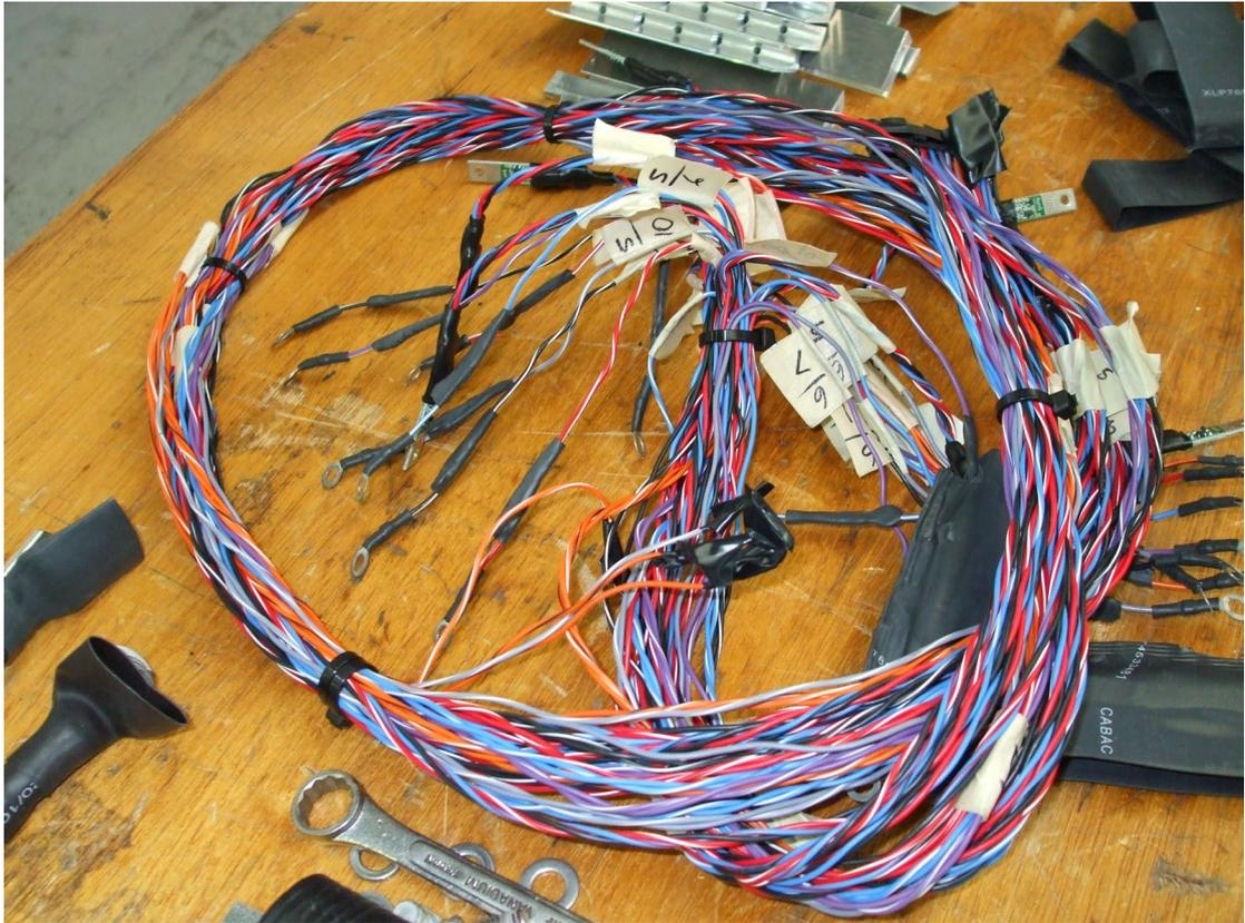
**Figure 7.12** The BMS wiring for half of the LiPo pack which is shown under construction in Figure 7.24.
