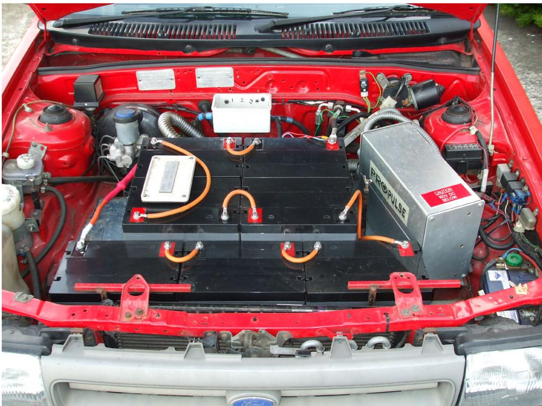
**Figure 6.3** EV conversion. A series string of 7 lead acid modules of 12 V each giving 84 V between the front and rear terminals. This arrangement, without terminal insulators, could conceivably be short circuited by somebody jumping on the bonnet of the car. The hazardous voltage (by some definitions) is also accessible without the use of tools.
