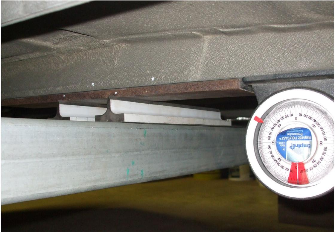
**Figure A7.2** Vehicle balanced on knife edges. Protractor with 0.5° accuracy shown.
