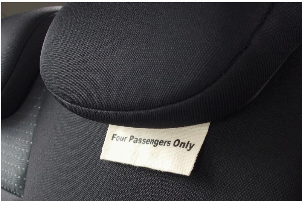
**Figure 8.3** Rear centre seat label fitted to Blade Electron Mk III.
