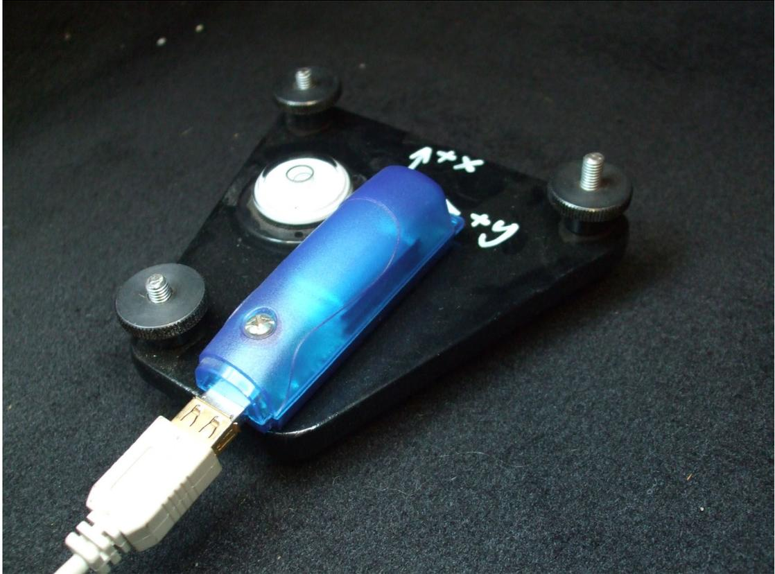
**Figure 8.13** X6-2 accelerometer mounted to the floor of a test vehicle.
