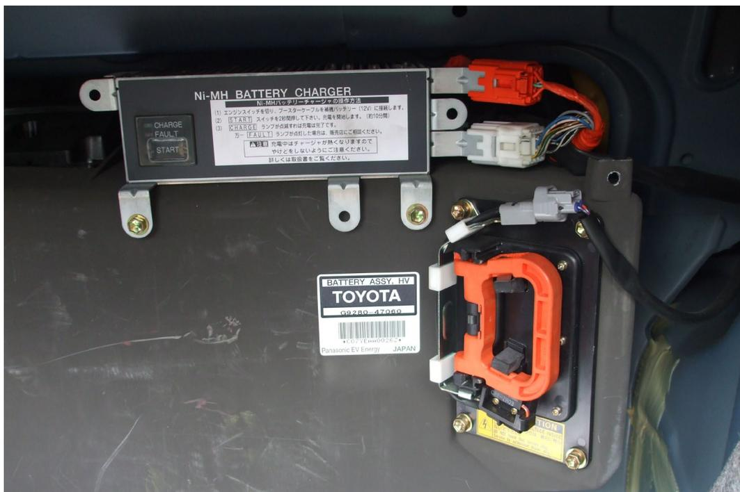
**Figure 6.5** 1999 Toyota Prius manual HV disconnect located in the boot of the vehicle.
