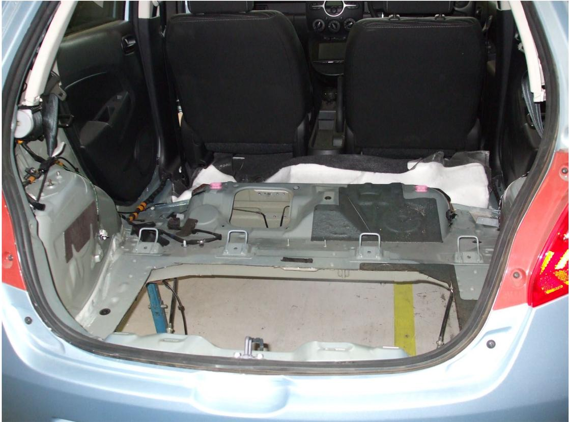
**Figure 7.21** The boot floor of a hatch cut-out either side of the chassis rails to allow a LiPo pack to be partially recessed.
