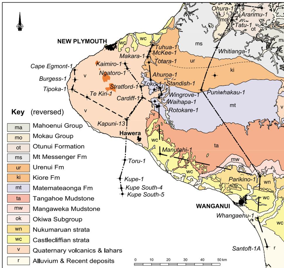
Fig.4. Geological map of central-western North Island including Taranaki Peninsula, showing the location of key hydrocarbon exploration holes and the line of four cross-sections.
