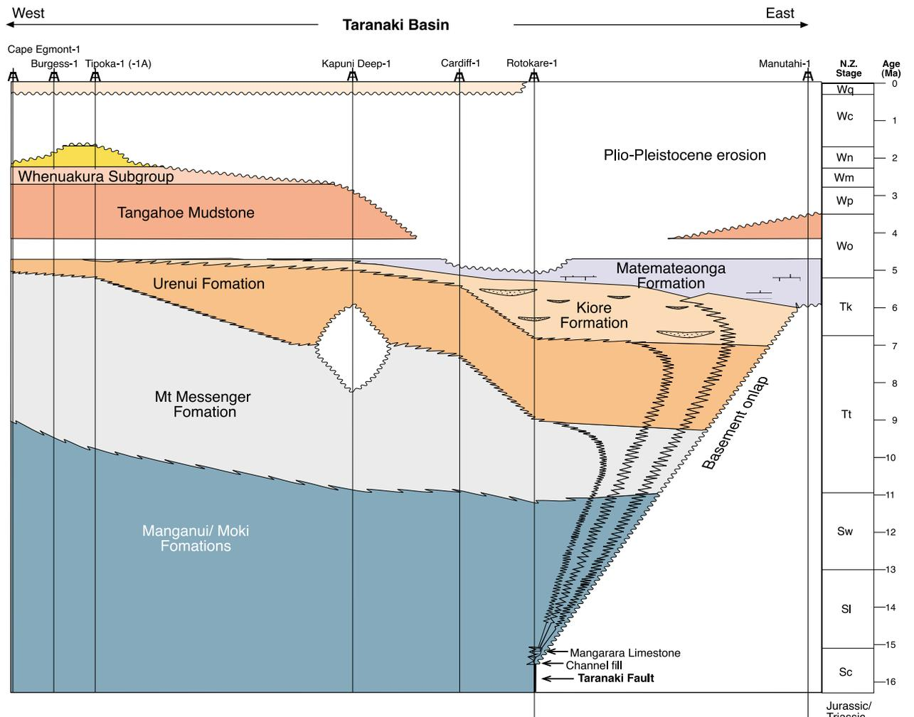
Fig.7. Taranaki Peninsula (Cape Egmont-1 to Rotokare-1) stratigraphic panel built up from well-to-well correlations, and related time-stratigraphic cross-section (extended to Manutahi-1).
