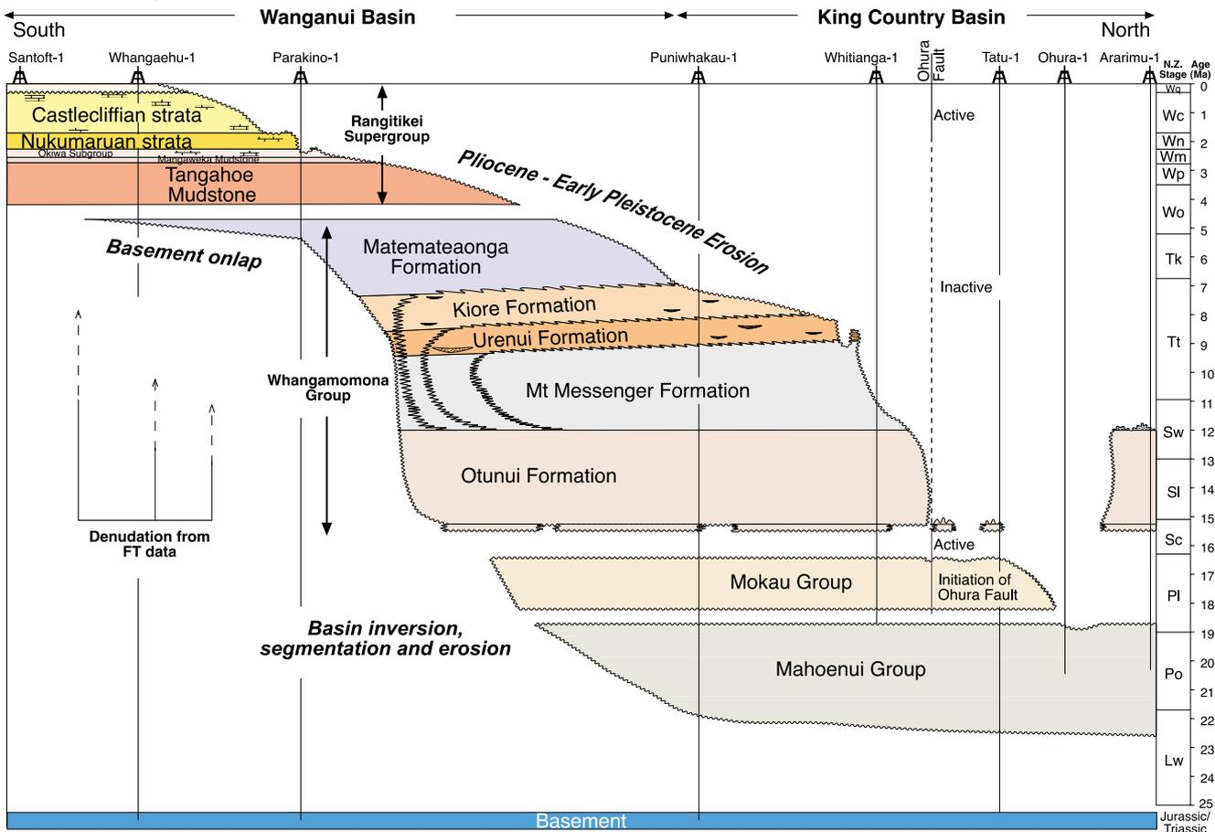
Fig.6. Wanganui Basin to King Country Basin (Parakino-1 to Ararimu-1) stratigraphic panel built up from well-to-well correlations, and related time-stratigraphic cross-section.
