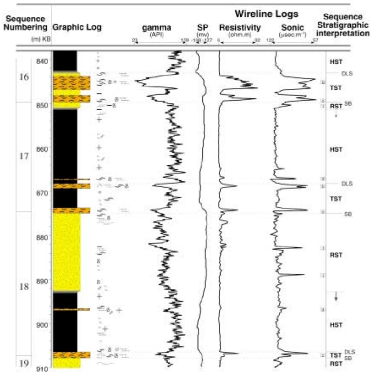
Figure 11: Stratigraphic and wireline log detail for sequences 16 to 19 in Manutahi-1, also showing the extent of systems tracts.
