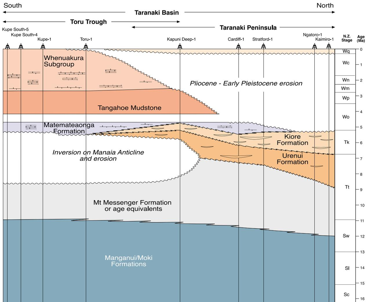
Fig.8. Toru Trough to Taranaki Peninsula (Kupe South-5 to Kaimiro-1) stratigraphic panel built up from well-to-well correlations, and related time-stratigraphic cross-section.
