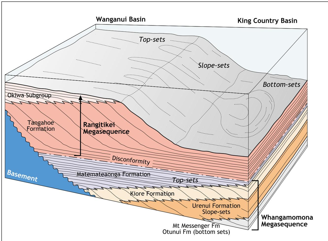
Fig.9. Block diagram showing schematically the occurrence of two continental margin wedges representing the Whangamomona and Rangitikei megasequences, each having prograded northward through central-western North Island during the late Neogene.
