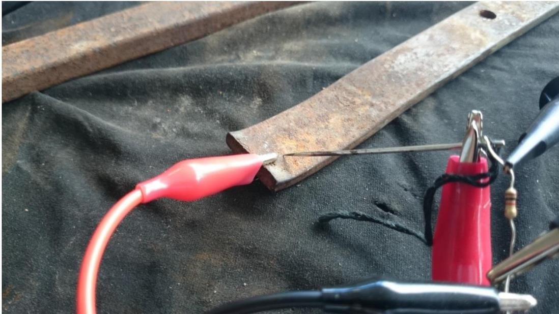
**Figure 48 – Corroded Joint Simulator. A steel needle is used to form one electrical connection to the junction while the electrical connection through the crocodile clip forms the other**
