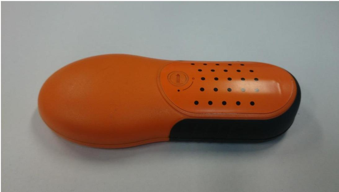
**Figure 24 – Gallagher iSeries Remote. Conductive plate is insulated by an orange sticker over the battery cover with black dots highlighting the area**
