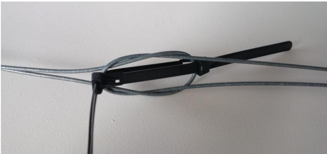
Figure 14 - Fence wire joined using reef knot
