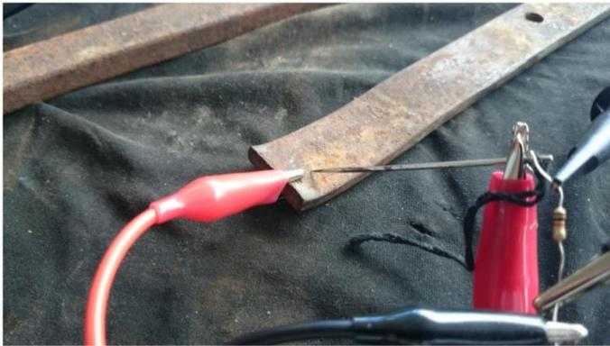
Fig. 2. Photo showing experimental setup of Rust Joint
