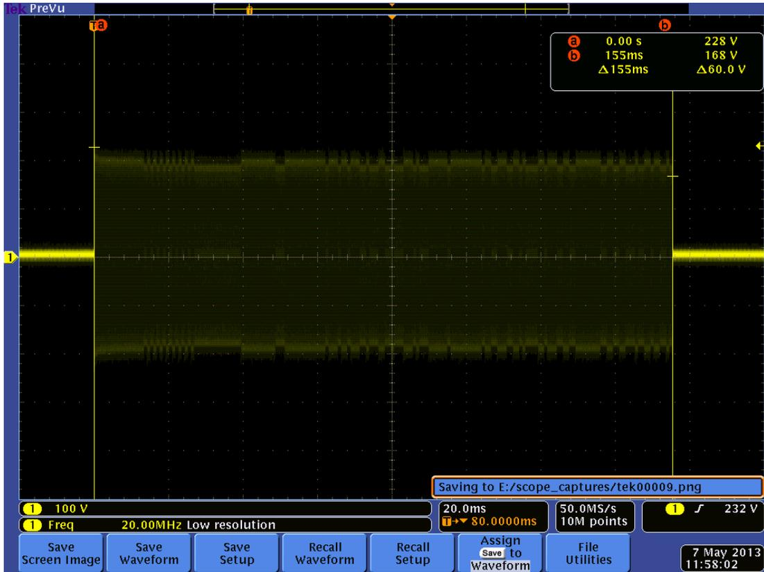
Figure 53 – Capture of a data transmission on a Gallagher fence. Figure shows an entire capture of an ON transmission, length approximately 155 ms. The various parts of the transmission can be distinguished such as the preamble and the main message
