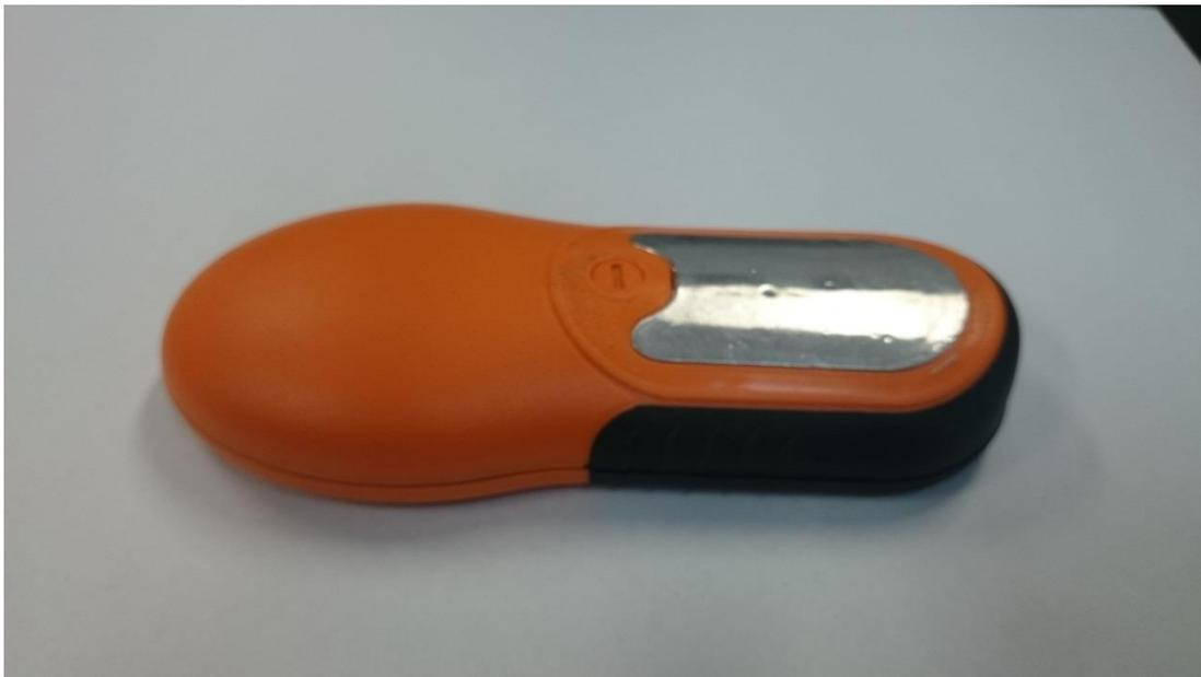
**Figure 27 - Gallagher iSeries Remote with insulating sticker removed from battery cover**
