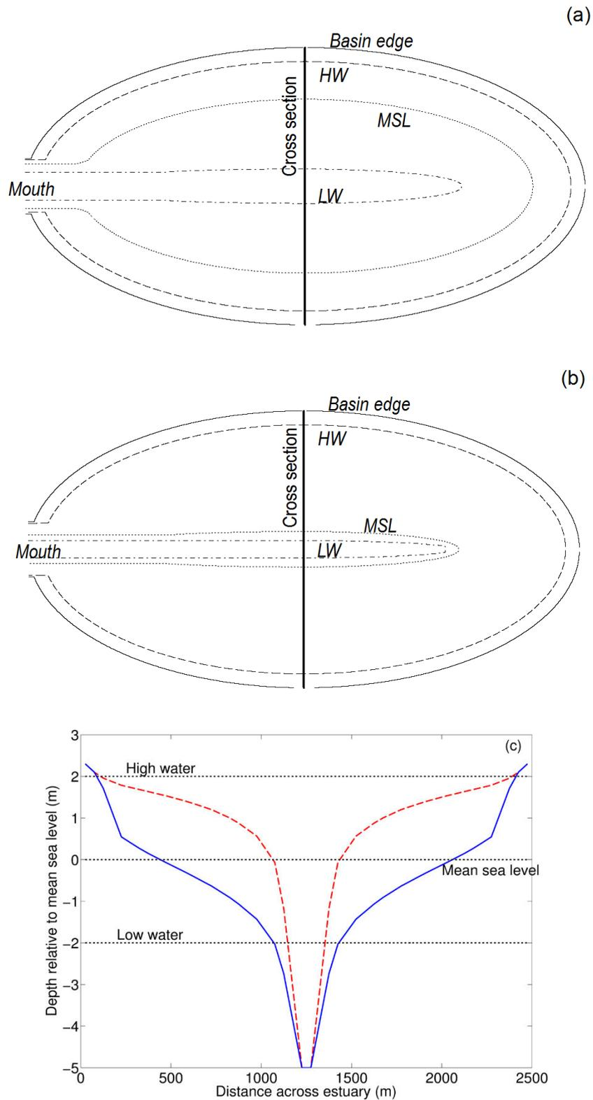
Figure 2.3. Schematic of unfilled (young) (a) and infilled (mature) (b) idealised morphologies showing location of LW, MSL and HW with cross sections taken through centre of basin (c) for unfilled (solid line) and infilled (dashed line) basins.
