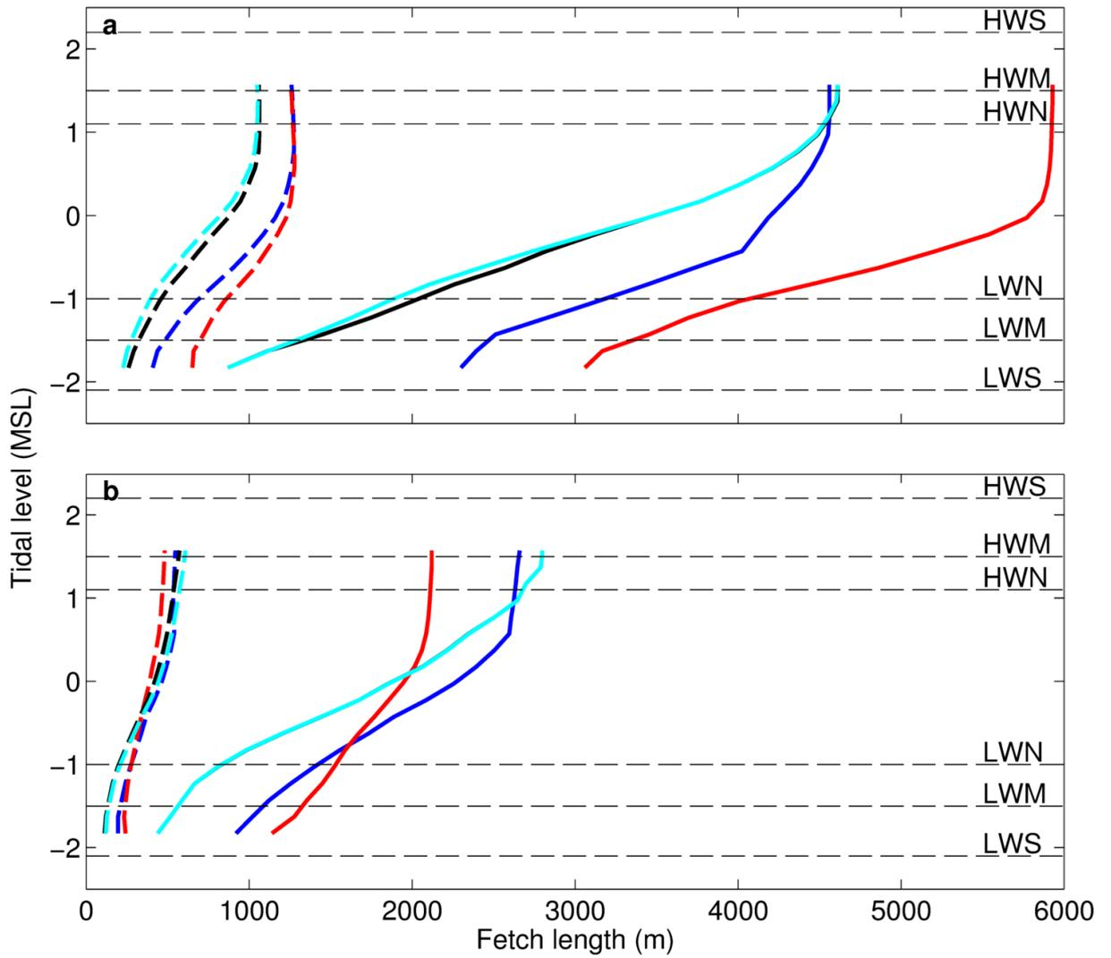
Figure 4.3: Fetch distribution with depth within the northern (Waingaro) arm (a) and the southern (Waitetuna) arm (b) for wind directions of 80° (blue line), 235° (red line), 135° (black line) and 315° (cyan line). Solid lines show maximum fetch within each basin and dashed lines show average fetch over entire basin. Horizontal dashed lines show tidal heights in Figures 4.4, 4.5 and 4.6.
