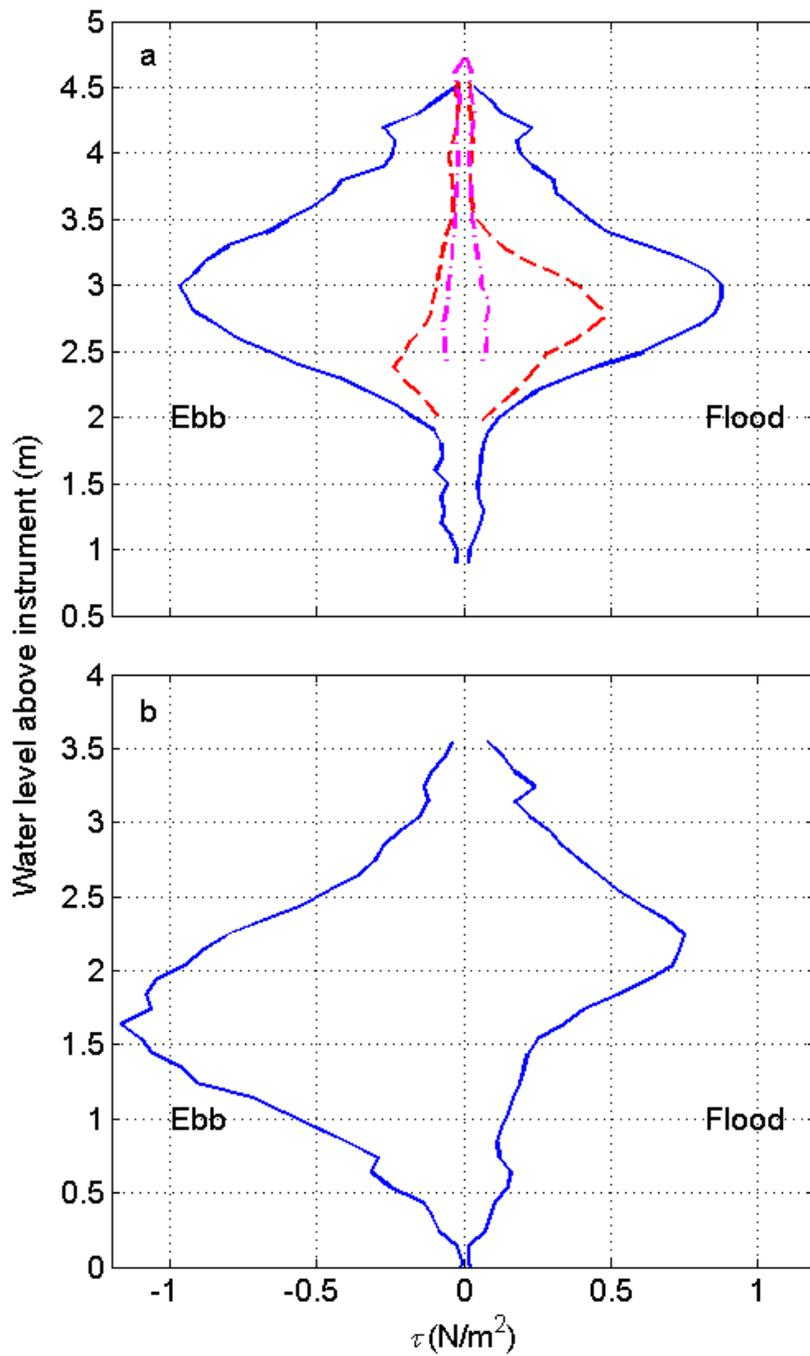
Figure 3.4: Tidal stage figures showing  $\tau$  (bin averaged over entire deployment, with 0.1 m vertical resolution) plotted for each water level for the northern arm (a): Acoustic Doppler Profiler (solid line), T1 (dash-dotted line) and T2 deployments (dashed line); and the southern arm Acoustic Doppler Velocimeter (b).
