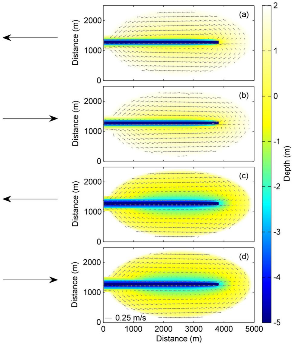
Figure 2.6. Depth-averaged flow residuals during a steady high-water level (no tide) with a spatially uniform and consistent 10 m/s seaward (easterly) (a and c) and 10 m/s landward (westerly) wind (b and d) for an infilled (a and b) and unfilled (c and d) morphology. Large arrows denote direction of wind.
