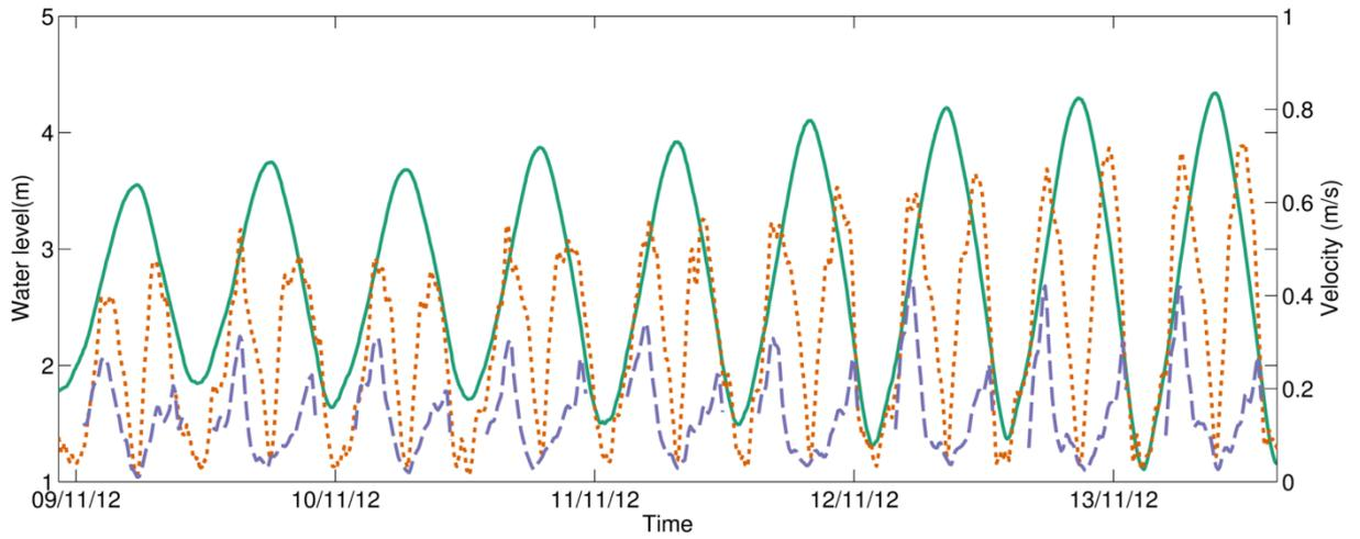
Figure 2.12. Water levels (solid line) and current velocities (dotted line) collected using a Sontek ADP (subtidal) and current velocities (dashed line) collected with a FSI 3DACM Wave recorder showing contrasting tidal asymmetries over the intertidal and subtidal areas of the northern (Waingaro) arm of Raglan Harbour, New Zealand. The locations of deployments are shown in Figure 2.4b
