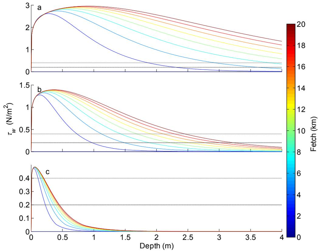
Figure 4.10: Calculated values of  $\tau_w$  for a range of fixed water depths and fetches for a strong (10 m/s, a), a moderate (5 m/s) and a weak (2 m/s, c) wind speed. The horizontal black dashed and dotted lines represent approximate maximum basin-averaged values of  $\tau$  in the subtidal channel during a spring and neap tide from the Raglan Harbour numerical model. Note the change in y-axis scale between a, b and c.
