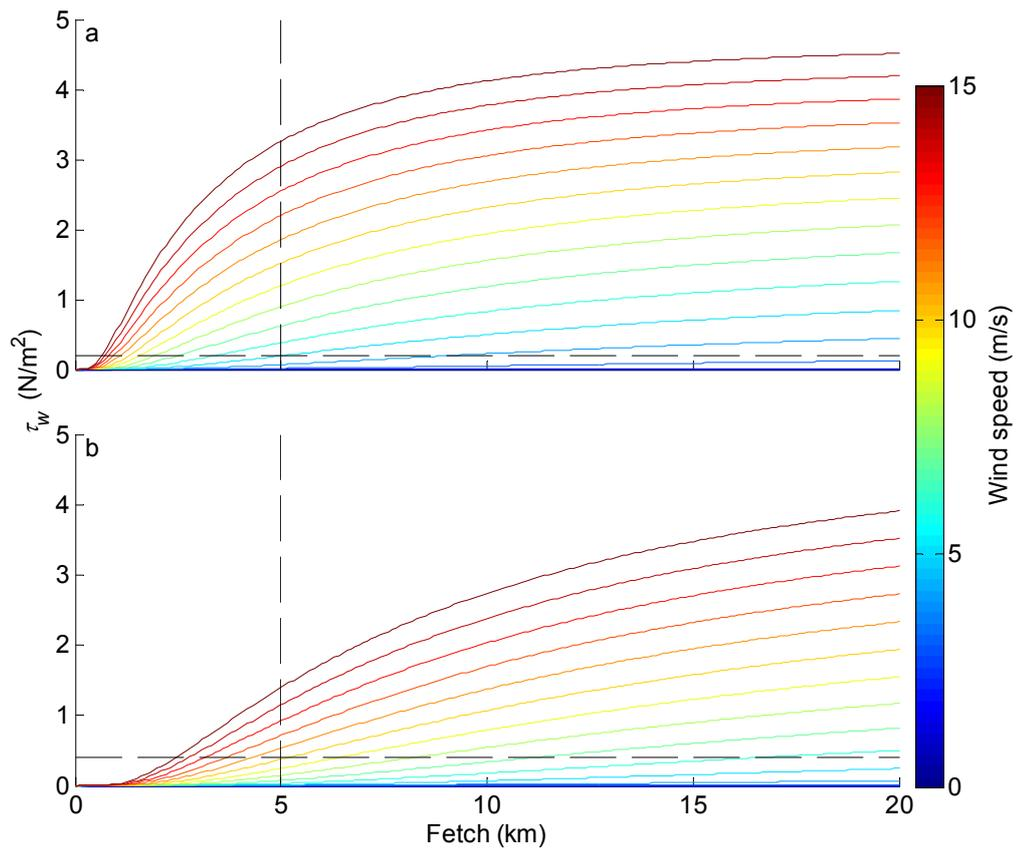
Figure 4.8: Values of  $\tau_w$  for a range of wind speeds and fetches for a single fixed typical neap (1.5 m, a) and spring (3 m, b) water depth. The vertical black dashed lines represent maximum fetch length in the northern arm of the case study site. The horizontal black dashed lines represent approximate maximum basin averaged values of  $\tau$  in the subtidal channel from the Raglan Harbour numerical model.
