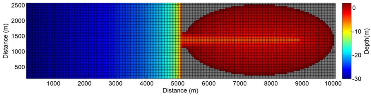
Figure 2.2. Numerical model grid and bathymetry. The model is forced at the single open boundary on the left hand side of the domain. The bathymetry in this figure is for the infilled basin ( $\gamma=4.0$ ).
