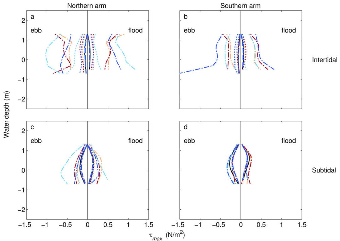
Figure 4.5: Tidal stage diagrams for a tide only scenario (black line), an 80° (orange line), 135° (dark red line), 235° (cyan line) and 315° (dark blue line) wind direction and a 2 (dashed lines), 5 (dotted lines) and 10 m/s (dash-dot lines) wind speeds. The tidal state shown here is for a single neap tidal cycle. The level of  $\tau$  is averaged over the intertidal (a) and subtidal (c) in the northern (Waingaro) arm and the intertidal (b) and subtidal (d) in the southern (Waitetuna) arm.
