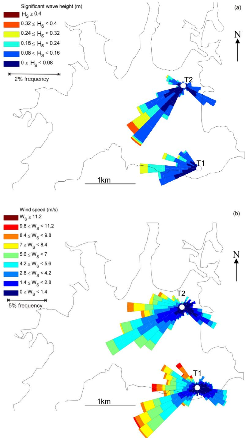
Figure 3.6: Panel a shows significant wave height (denoted by the colour) and frequency of occurrence (denoted by the length of each column relative to the scale bar) for each Dobie deployment. The direction of wind blowing during each wave event is taken from the Raglan weather station and is shown by the orientation of each column. Panel b shows the magnitude, frequency and direction of wind recorded at the Raglan weather station during each deployment.
