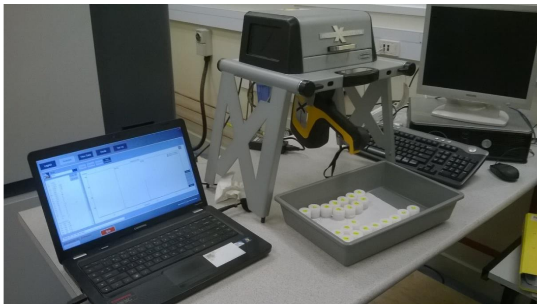
Figure 5-5 Laboratory setup of the handheld XRF showing the standard operational setup of the four main components (laptop, samples, bench-top, and XRF).
