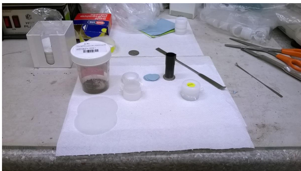
Figure 5-4 Sub-sampled 2 mm fraction is prepared into an XRF sample container for elemental analysis.
