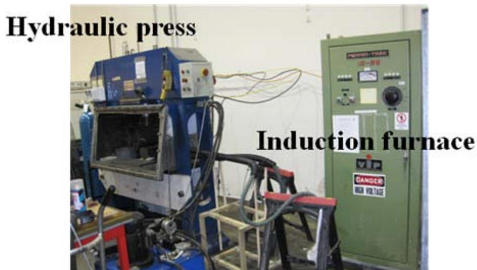
Figure 2.3: 100-ton hydraulic press and induction furnace.
