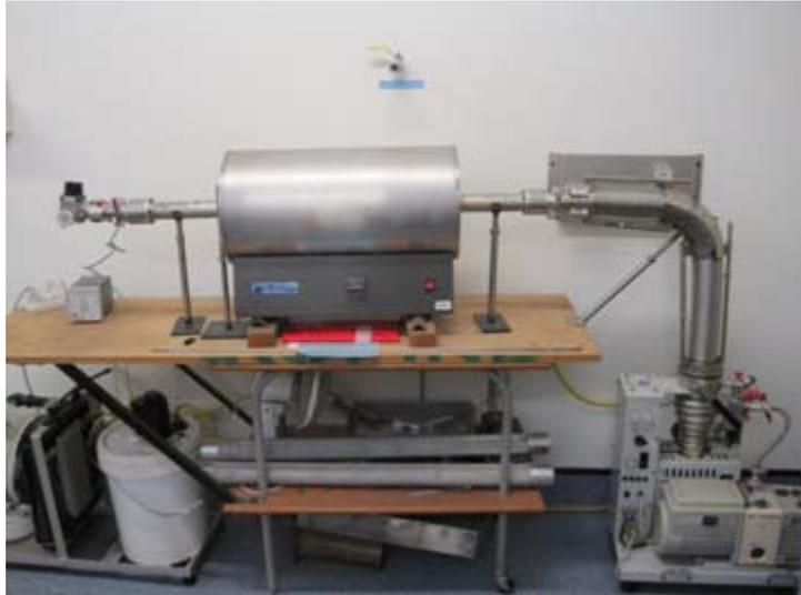
Figure 2.2: Stainless steel vacuum tube furnace.
