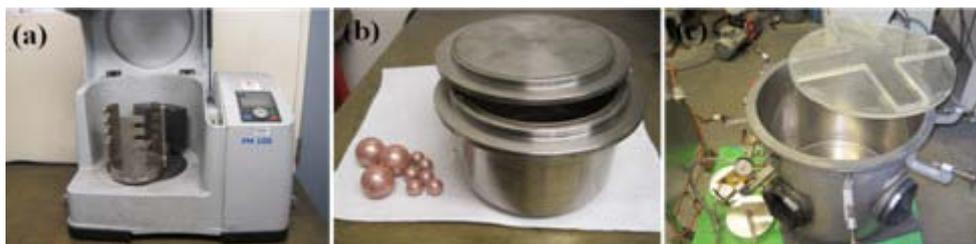
Figure 2.1: (a) Retsch PM100 planetary ball mill; (b) steel vial and stainless steel balls with diameters of 12.5 and 25 mm; (c) glove box.
