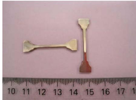
Figure 2.5: Tensile specimens cut from extruded Cu-5vol.%Al<sub>2</sub>O<sub>3</sub> composite rods.
