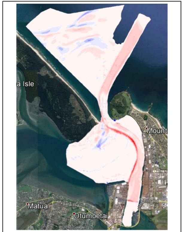
**Figure 10.** Comparison of MBES surveys before and after dredging: red indicates erosion and blue indicates accretion (Thomas Saillour).
