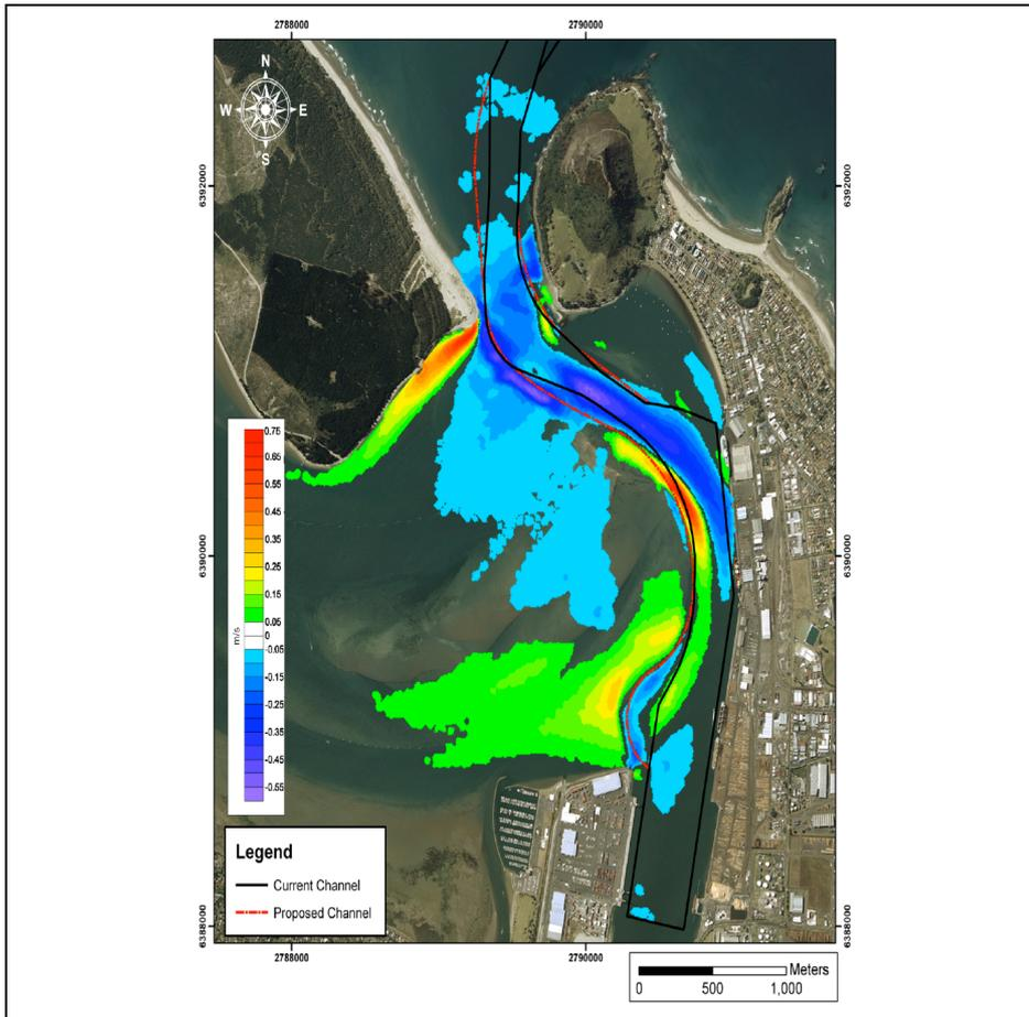
**Figure 6.** Predicted change in peak spring flood tide velocities following completion of all proposed dredging (Figure 9.61 – Healy Evidence): positive values indicate an increase in velocity after dredging.
