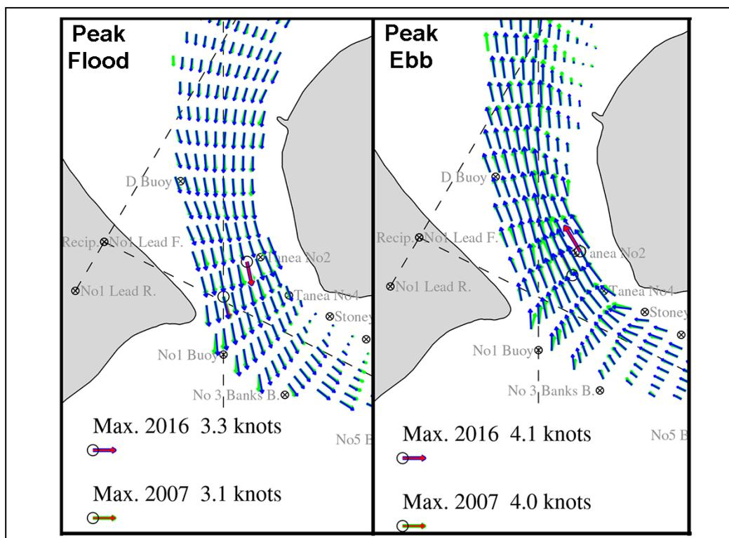
**Figure 9.** Comparison of spring tide peak flood and ebb flow velocities through the tidal inlet measured by ADCP surveys in 2007 (green) and 2016 (blue). (Taken from pages 4 and 5 of Vennell, 2017).
