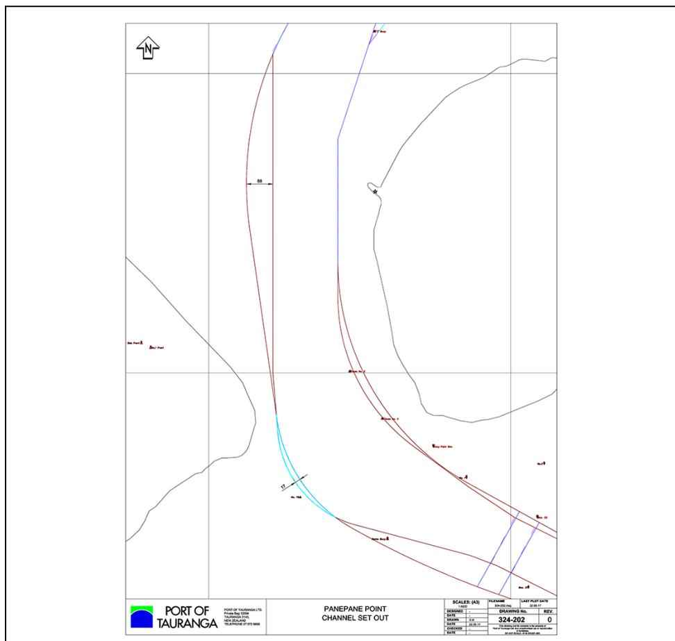
**Figure 5.** Summary of the changes to the channel alignments through the tidal inlet of Tauranga Harbour. (Port of Tauranga drawing No 324-202)
