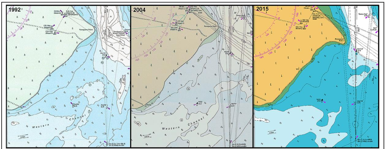
**Figure 2.** Sections of LINZ hydrographic chart NZ 5412 – Port of Tauranga – highlighting Panepane Point and the Lower Western Channel shoreline of Matakana Island. The charts show the south-eastward extension of Panepane Point associated with erosion to the south forming a more prominent spit, and shoaling of the Lower Western Channel.
