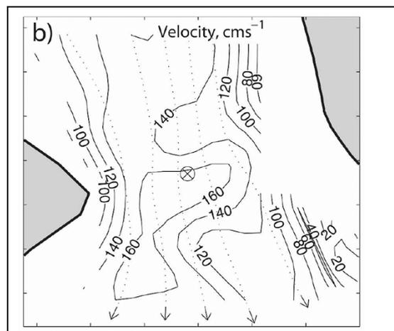
**Figure 4.** Peak flood depth-averaged velocity in the Tauranga Harbour entrance measured by a boat mounted ADCP in January 1993 (Figure 4b, Vennell, 2006).
