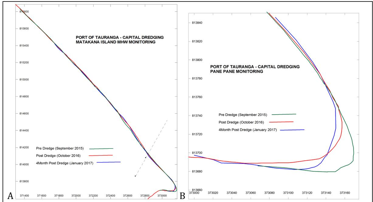
**Figure 8.** Summary of mean high water mark (MHW) surveys of southeastern Matakana Island conducted by the Port of Tauranga before and after the 2015-16 capital dredging (A), including an enlargement of the Panepane Point section (B). Note the September 2015 survey on the diagrams was undertaken in August 2015. (Drawings provided by DML)
