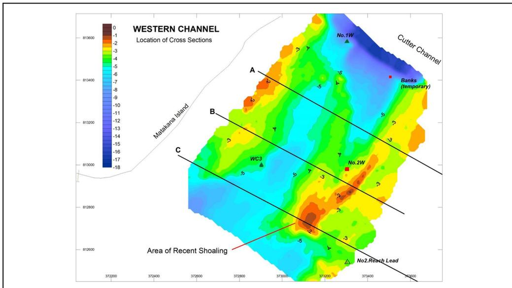
**Figure 11.** Bathymetry of the Lower Western Channel obtained by the Port of Tauranga in July 2016. The cross-sections marked correspond to those in Figure 12.
