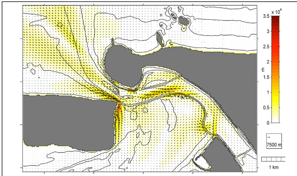
**Figure 7.** Full spring tide residual differences between pre and post-dredging model results. The arrows indicate the magnitude and direction of sediment transport, and the colour contours also indicate the magnitude of transport. (Figure 9.70 Healy Evidence)
