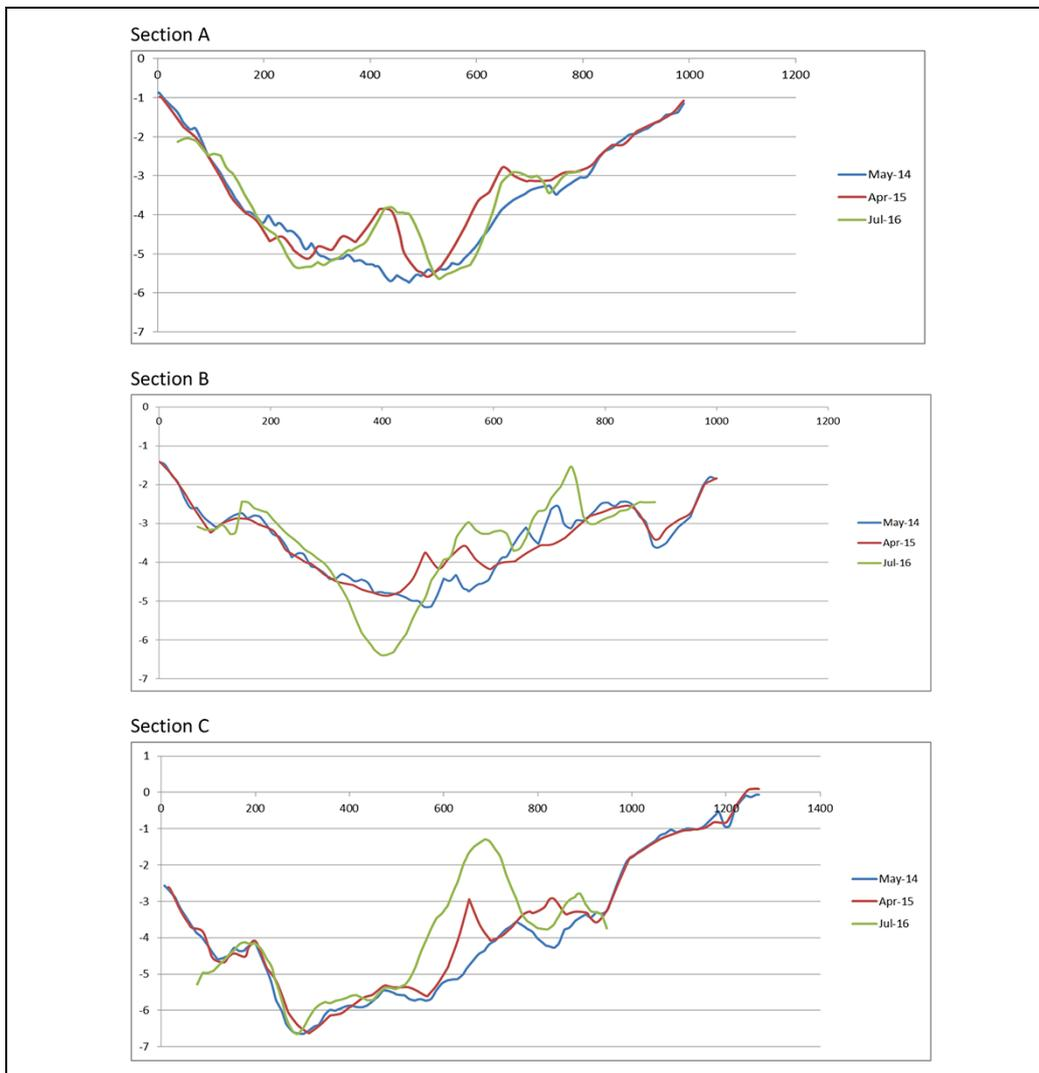
**Figure 12.** Comparison of cross-sections of the Lower Western Channel 2014-2016.
