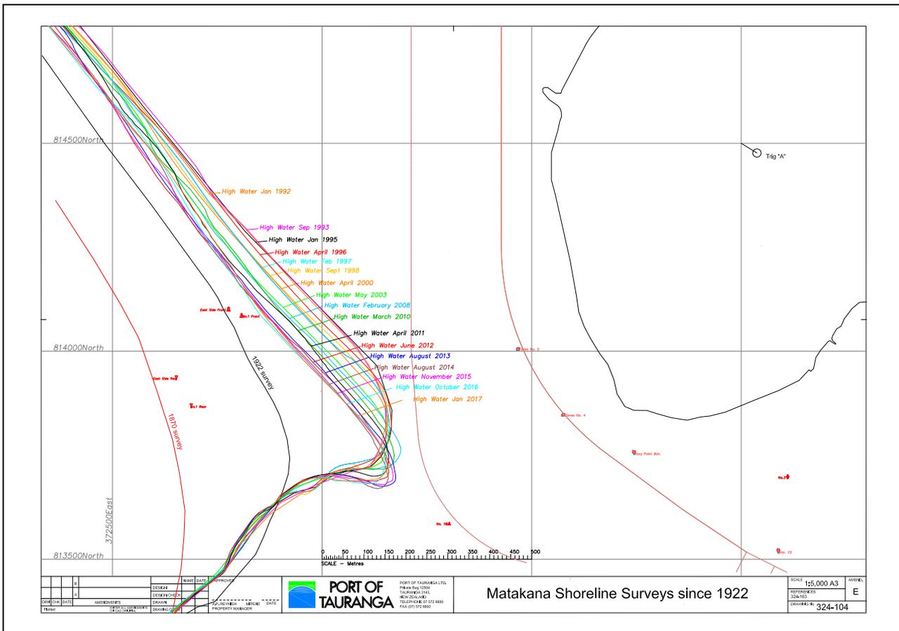
**Figure 3.** Summary of mean high water mark (MHW) surveys of southeastern Matakana Island conducted by the Port of Tauranga since 1992 compared to the 1922 reference shoreline. (Port of Tauranga drawing No 324-104)
