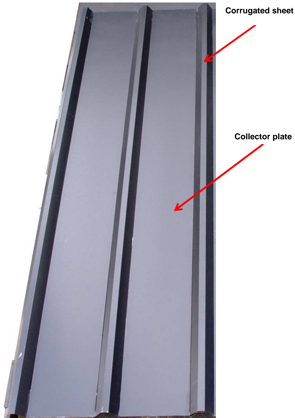
Figure 4.5 Prototype comprising corrugated sheet with collector plate made from Colorcote steel.
