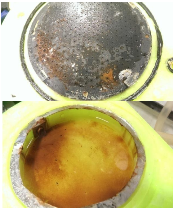
Figure 4.12 Corrosions inside the PEFT cell
