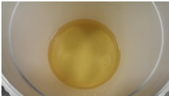
Figure 4.13 Yellowish color solution resulted in after current flowed through electrodes
