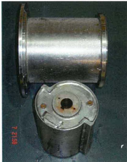
Figure 3.3 Step rotor and screen cylinder.
