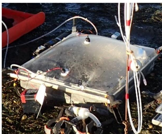
Figure A1.2. Large custom benthic incubation chamber (Kaipara Harbour, 2016).
