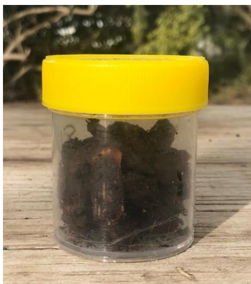
Figure 3.6: Example 70 mL specimen vial \frac{3}{4} filled with bark
