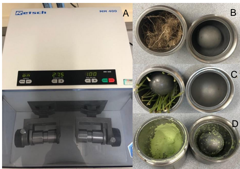
Figure 2.6: Procedure for grinding plant material. A) Ball mill, B) Root material prior to grinding, C) Pseudostems prior to grinding and D) Pseudostems post grinding
