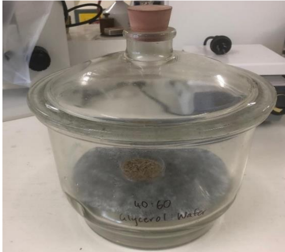
Figure 2.1: Seed set up (in 60 mm Petri dish) in desiccator containing glycerol and water for accelerated aging
