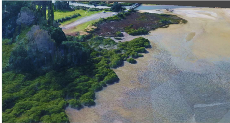
Figure 5.20. Point cloud model from a fixed-wing RPA photogrammetry flight near Waiponga Reserve, Wharekawa Harbour on 25 May 2017 (3-D scene perspective in Agisoft Photoscan 1.5) showing vertical structure running from high variability at the coastal margin (mangrove, marsh and saltmarsh ribbonwood / manuka, then dune grass community types running from lower left to upper middle), with dense seagrass (lower right) blending up to and into the mangrove margins.
