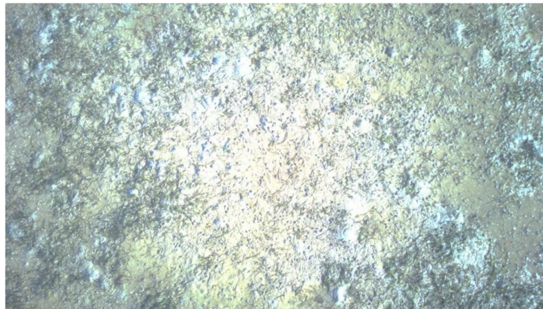
Figure 2.4. An example of vignetting (radial attenuation) in a raw sensor image (Nokia Lumia 1020 camera) elevated at 5m height over a patch of seagrass.
