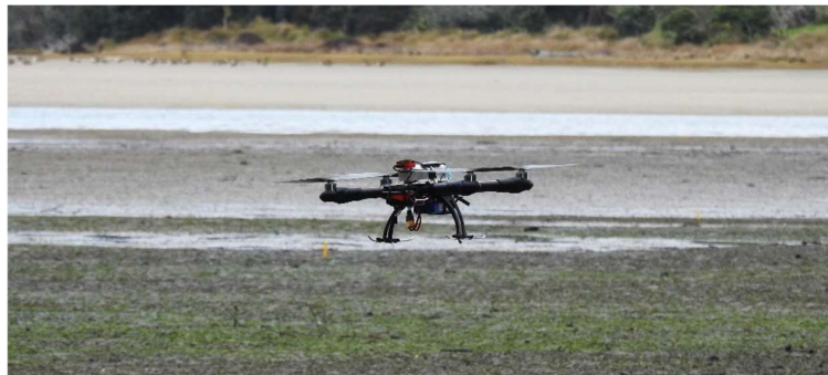
Figure 4.3. Camera drone in flight over seagrass meadow; multispectral camera with downwelling sunlight sensor mounted at front.
