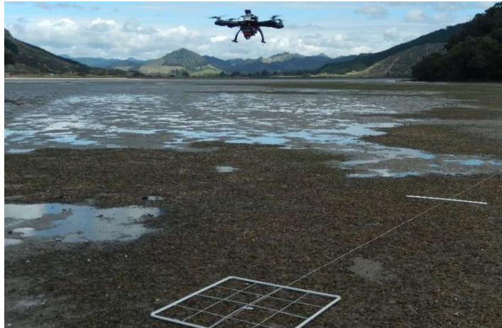
Figure 7.1. An RPA flying under GPS guidance can target specific sampling points along programmed routes as a ‘mobile quadrat’. In the case below the RPA is flying along a reference transect for calibration purpose. Fitted with RTK-GNSS guidance and gimbal control of camera orientation, decimetre positional accuracy of image contents is feasible.
