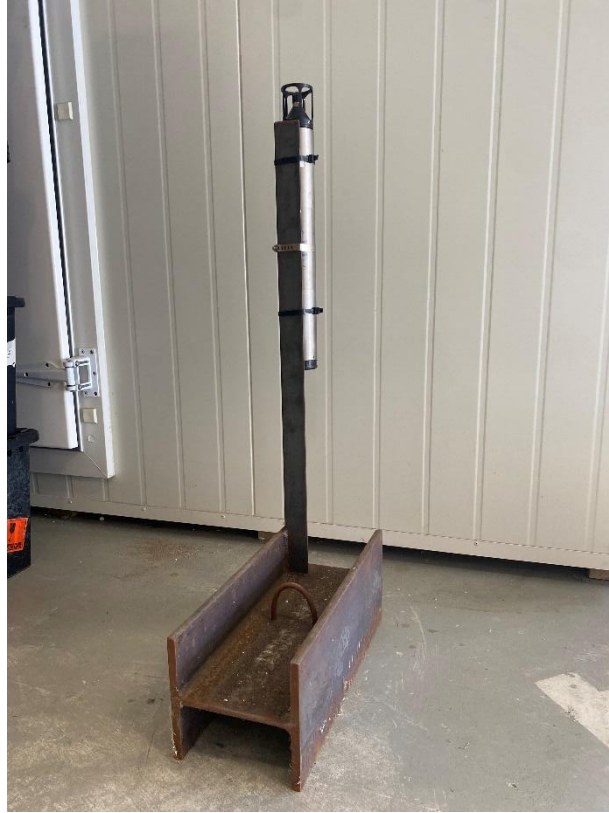
Figure 4. Photograph of mooring configuration with weighted stand and attached SoundTrap 600 in the laboratory.
