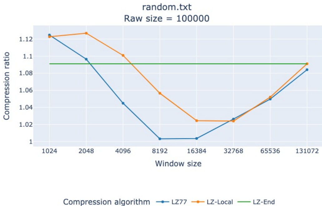
Figure 7.15: A random file will not compress; however, the graph shows that a larger window size does limit the number of LZ-Local phrases, reducing its compression ratio. This continues until a window size of 32768, after which larger window sizes increase the phrase size without effectively reducing the number of phrases into which the string is compressed.
