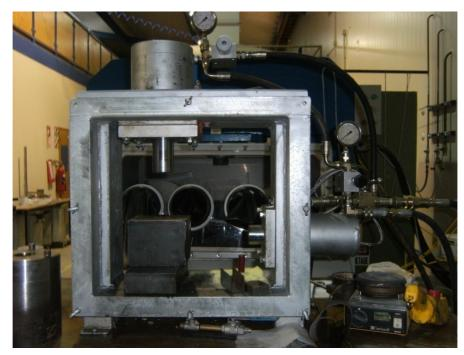
Figure 3.3 Hydraulic press and the rigid die used for the powder/spacer material mixture.
