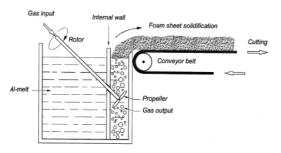
Figure 2.5 Direct foaming of melts by gas injection [9].
