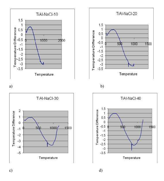
**Figure 4.2** DTA results of TiAl powder blended with NaCl spacer material. (a) 10%V of NaCl spacer material, (b) 20%V of NaCl spacer material,(c) 30%V of NaCl spacer material, and (d) 40%V of NaCl spacer material
