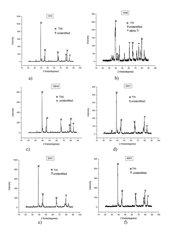
**Figure 4.3** XRD patterns of porous sample produced by *NH*<sub>4</sub>*HCO*<sub>5</sub> spacer material with different volume percentage, a) 10H1, b) 10H4, c) 10H6, d) 20H1, e) 30H1, and f) 40H1
