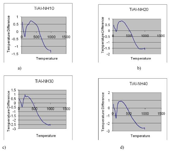
**Figure 4.1** DTA results of TiAl powder blended with  $NH_4HCO_2$  spacer material. (a) 10%V of  $NH_4HCO_2$  spacer material, (b) 20%V of  $NH_4HCO_2$  spacer material, (c) 30%V of  $NH_4HCO_2$  spacer material, and (d) 40%V of  $NH_4HCO_2$  spacer material
