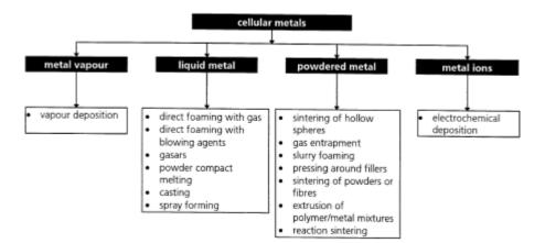
Figure 2.4 Leading production methods of the porous metals [9].
