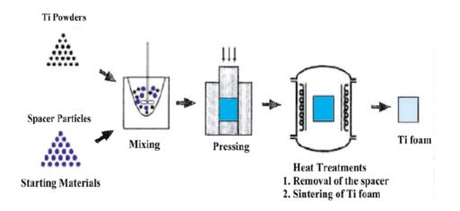
Figure 3.1 Pictorial representation of processing steps involved in production of porous TiAl.[2]
