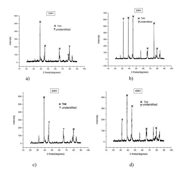
**Figure 4.4** XRD patterns of porous sample produced by NaCl spacer material with different volume percentage, a) 10N1, b) 20N1, c) 30N1, d) 40N1
