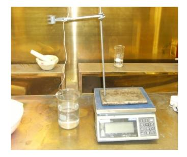
Figure 3.5 Set-up for density measurement.
