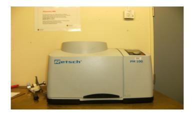
Figure 3.2 Retsch planetary ball milling machine.
