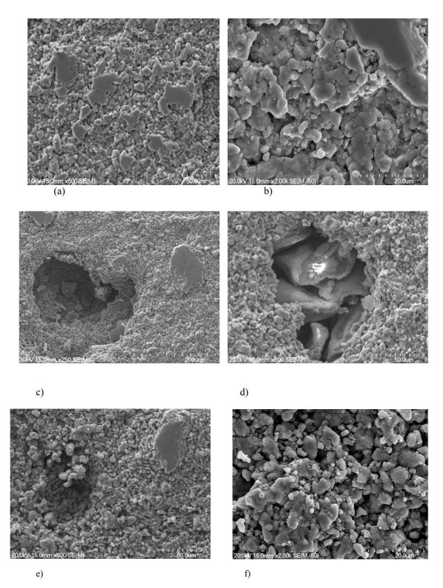
**Figure 4.10** SEM images of TiAl foams fabricated using different volume fractions of  $MH_{4}HCO_{4}$  spacer material (a) & (b) 20H1, (c) & (d) 30H1 and (e) & (f) 40H1.
