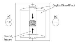
Figure 2.9 Schematic representation of FAST or EDC [10].
