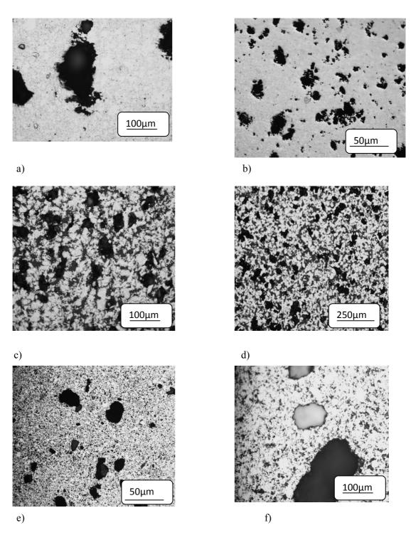
**Figure 4.5** Optical microscopy images of TiAl foams fabricated using  $MH_4HCO_2$  spacer material with and different sintering times; (a) & (b) 10H1, (c) & (d) 10H4 and (e) & (f) 10H6.
