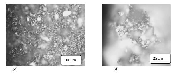
**Figure 4.8** Optical microscopy images of TiAl foams fabricated using different volume fractions of  $NH_4HCO_5$  spacer material (a) & (b) 30N1, (c) & (d) 40N1.
