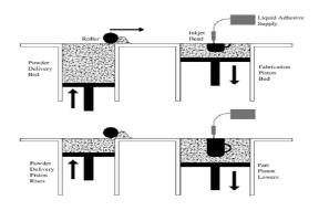
Figure 2.10 The use of 3DP process in fabrication of porous metals [10].
