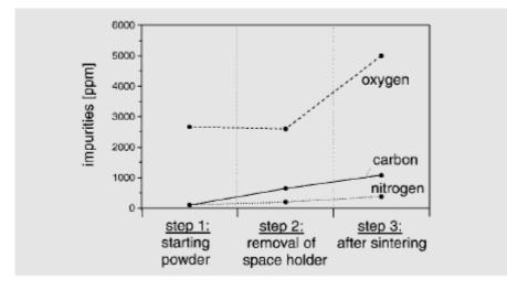
**Figure 4.12** Chemical analyses of oxygen, carbon, and nitrogen contents in titanium samples relative to processing steps [4]
