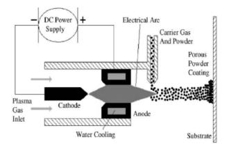
Figure 2.7 Schematic representation of plasma spraying process [10].
