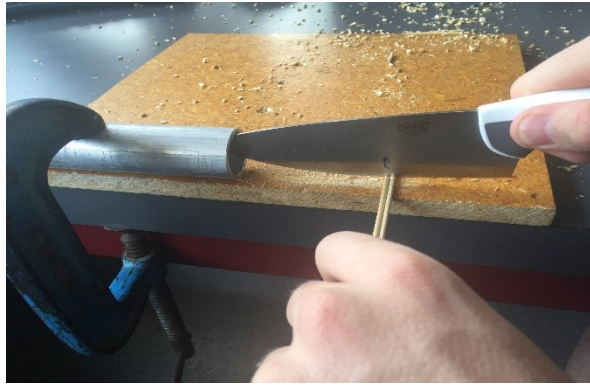
Figure 6 - Bamboo cutting technique with improvised blade tip holder allows more force to be applied while maintaining identical cutting motion between tests
