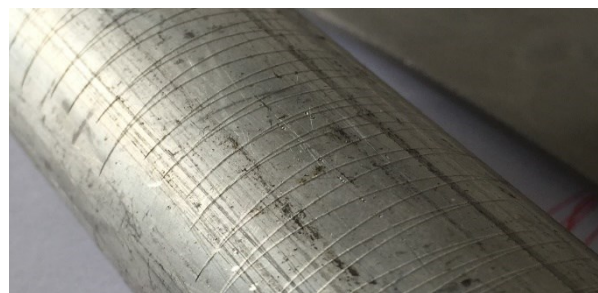
Figure 2 - Grooves formed in aluminium pipe diminish blunting capability
