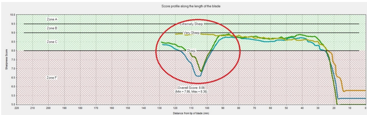
Figure 9 - Belt sharpened results showing 2.5 point drop in sharpness score after 60 cuts
