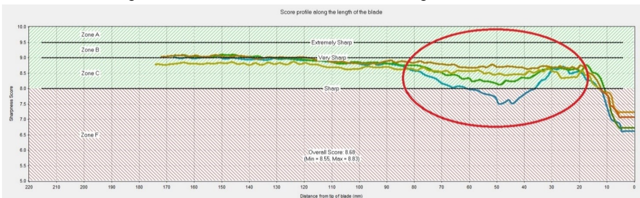
Figure 5 - Bamboo blunting tests show gradual blunting of edge through section used for cutting (circled)
