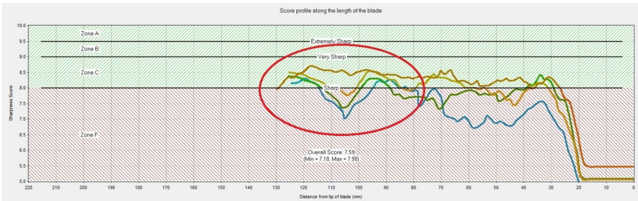
Figure 8 - Stone sharpened tests show a drop of 1.5 in the sharpness score after 90 cuts
