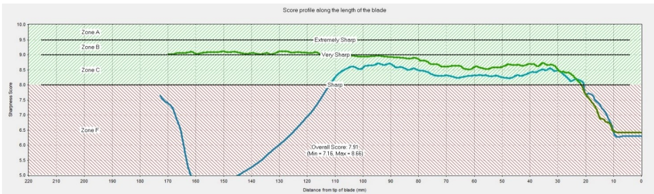
Figure 4 - Carbide emery paper results show edge is completely destroyed by only second test
