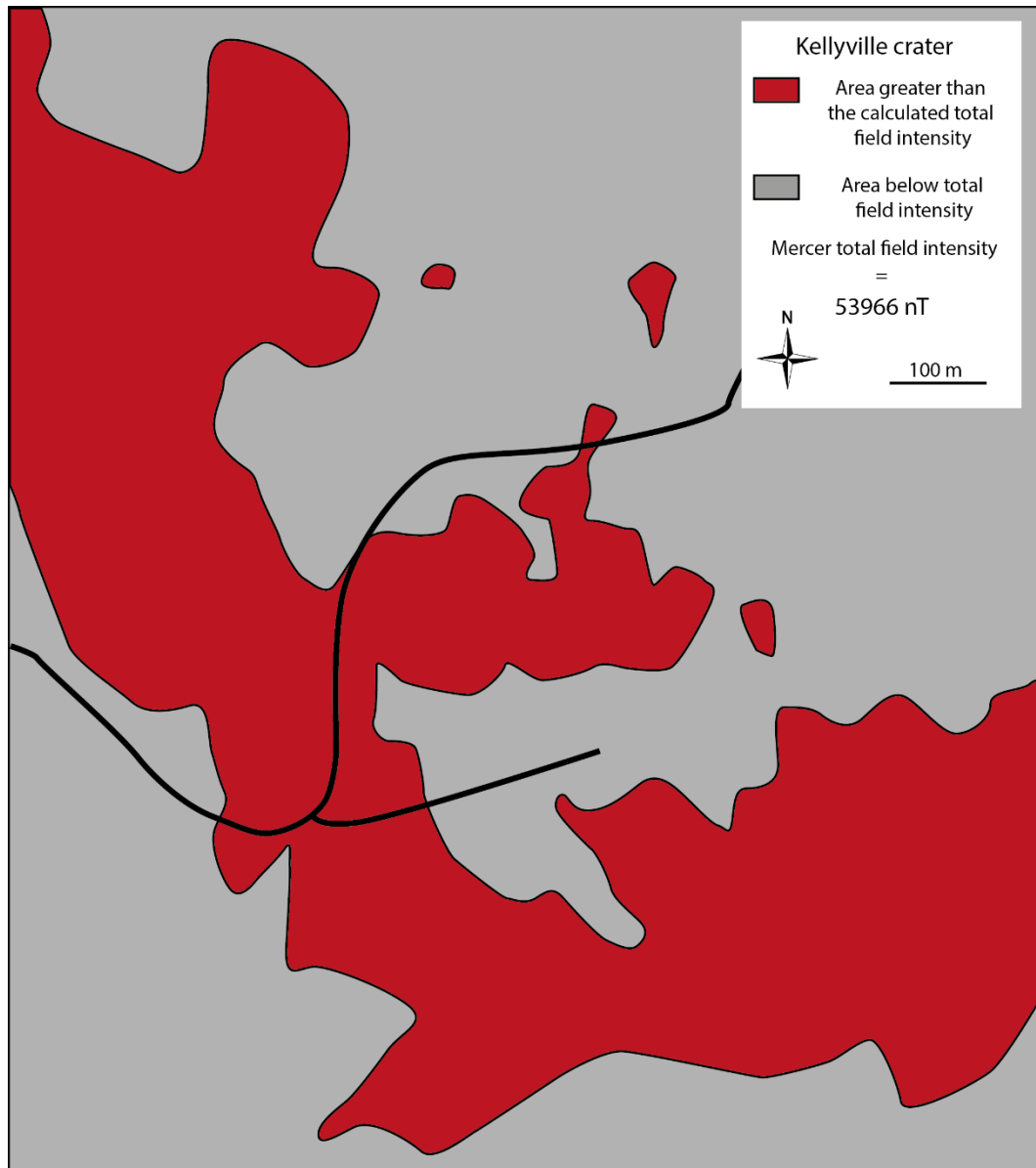
Figure 5.11: A map outlining the area in the Kellyville crater that is above what was calculated as the normal magnetic intensity for the Mercer region.
