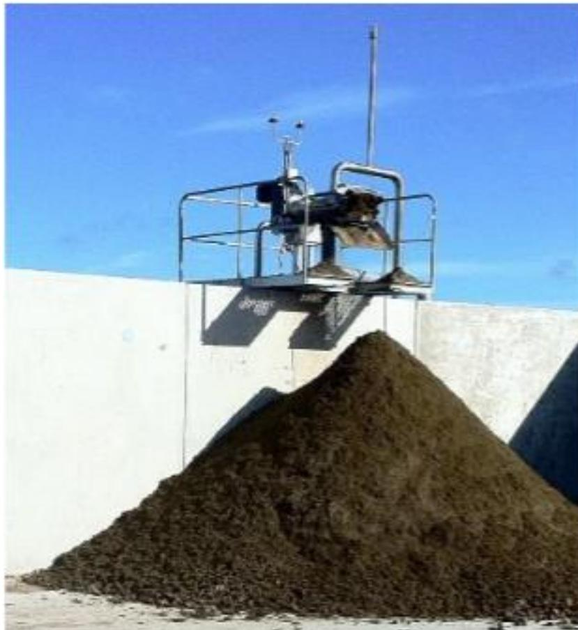
*Figure 2-11. Screw press separator (Dairy NZ, 2012).*
