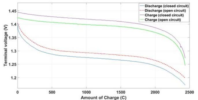
Fig. 5. Cycle test of 900mAh NiMH battery
