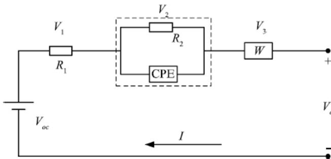
Fig. 4. Fractional equivalent circuit model reproduced from [12].
