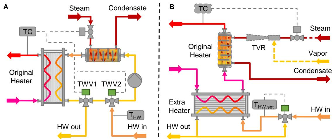
Figure 5: Hybrid Heating Systems. System A: HW-Integration into isolated HW-loop with three-way valves; System B: HW-Integration with additional Heat Exchanger.
