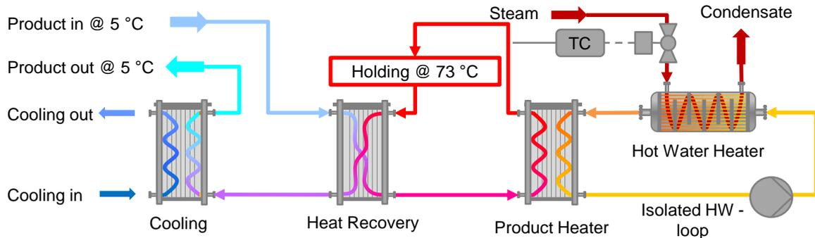
Figure 3: Pasteurization plant with heat recovery, heating and cooling section.
