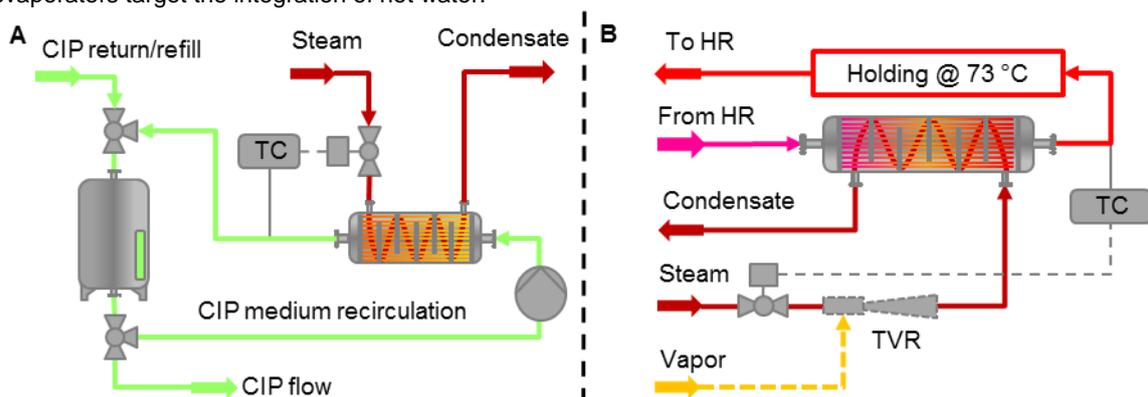
Figure 4: (A) CIP station; (B) Thermal treatment of evaporator feed, optional with TVR.
