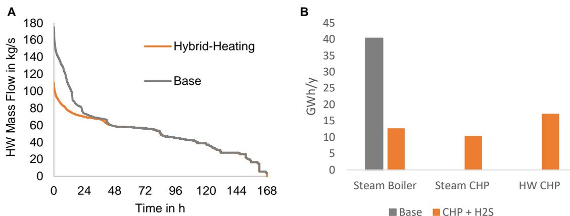
Figure 7: Results from the simulation. (A) Cumulative HW mass flows for the H<sup>2</sup>S compared to demand; (B) Comparison between steam supply only (Base) and the integration of a CHP unit and the H<sup>2</sup>S.
