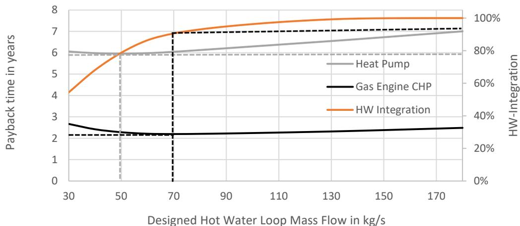
Figure 4: Correlation of designed HW-loop (incl. storage and CHP size adjusting), payback time, and the corresponding HW integration fulfillment.
