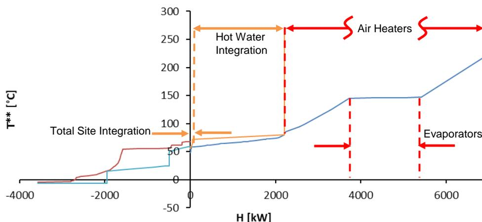
Figure 1: Total Site Profiles for the whey separation and drying process.
