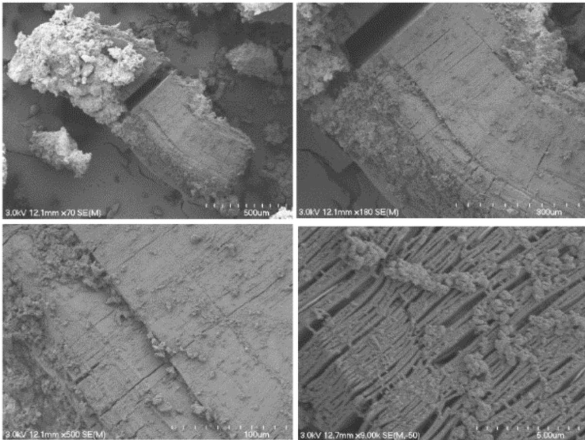
**Fig. 2.** SEM image of a giant, tightly laminated halloysite book (in two pieces) in ~930,000 year-old Te Puna tephra (Pahoia site, Tauranga). This book is ~1500 µm long (~1.5 mm). Enlargements of the book surface are shown, with increasing magnification, in images at top-right, bottom-left, and bottom-right. From Cunningham et al. (2016, p. 361).
