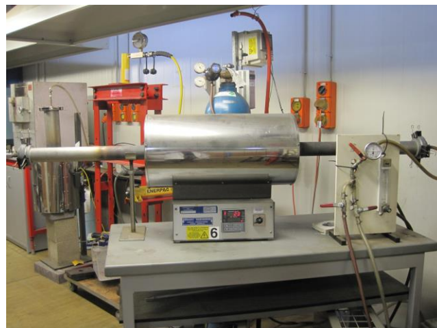
Figure 2.10 Horizontal tube furnace used for heat treatment.
