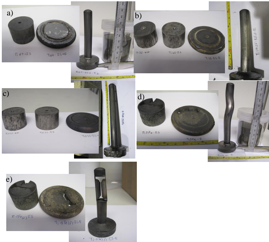
Figure 5.15 Images of a) Ti6Al4V, b) Ti3Al2V, c) Ti5SS, d) Ti5Fe-c, e) Ti5Fe-f alloys consolidated by forging or extrusion following IS-route.
