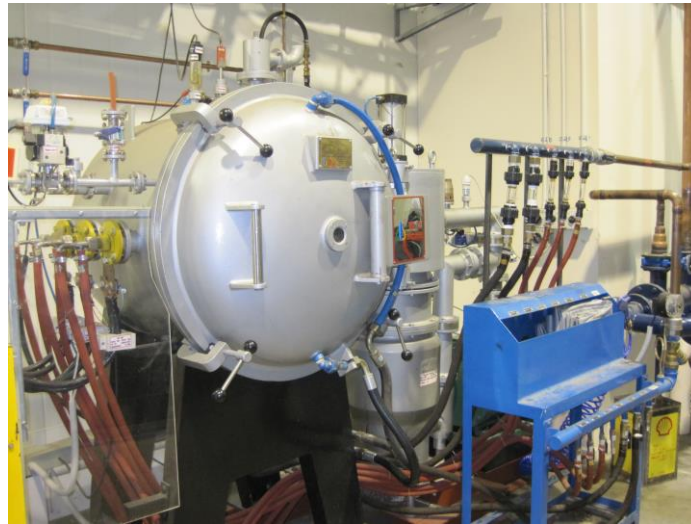
Figure 2.9 High vacuum furnace used for vacuum sintering.
