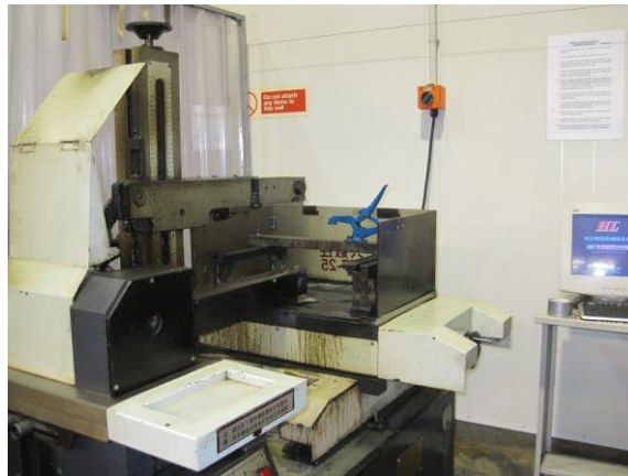
Figure 2.13 EDM cutting machine with a digital control.
