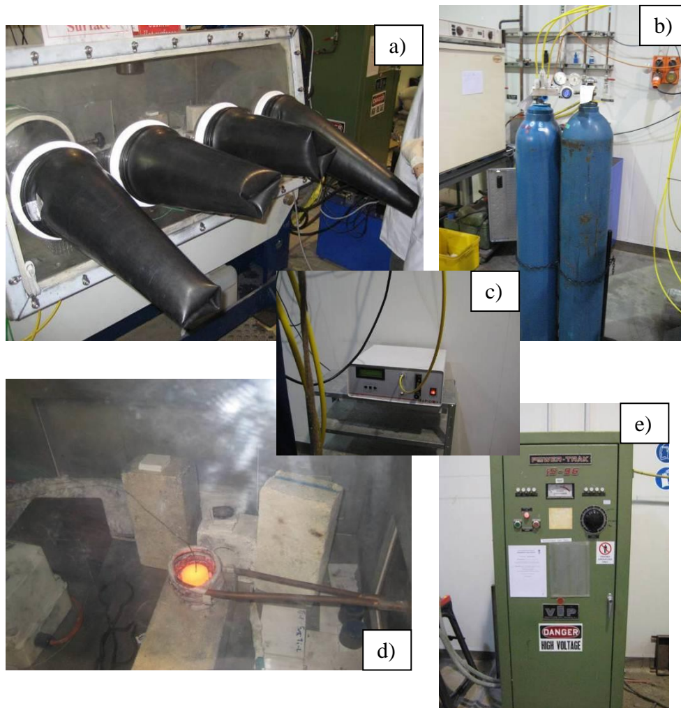
Figure 2.4 Experimental setup for induction sintering: a) controlled atmosphere chamber, b) argon bottles, c) oxygen analyser, d) induction coil mounted in a protective atmosphere chamber and e) induction power control unit.
