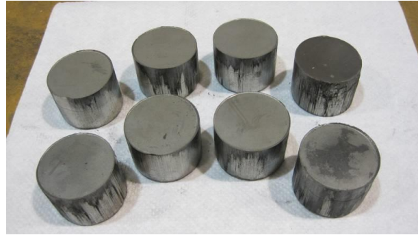
Figure 4.2 Images of Ti6Al4V alloy powder compacts.
