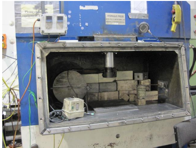
Figure 2.12 100 ton hydraulic press.
