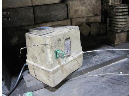
Figure 2.11 Thermocouple wire connected to a temperature controller.
