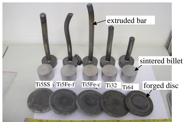
Figure 5.16 Images of Ti6Al4V, Ti3Al2V, Ti5SS, Ti5Fe-c and Ti5Fe-f alloys consolidated by forging or extrusion following VS-route.
