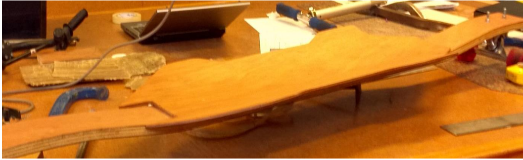
Figure 5.5 Positioning of the body pan on a wooden frame (lowered to the ground).
