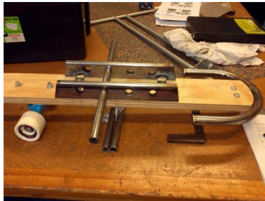
Figure 5.16 MY's adjustable footrest, achieved through problem solving and interaction with the luge components.
