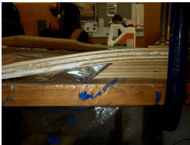
Figure 5.10 Laminated sheets of plywood to make the wooden frame.
