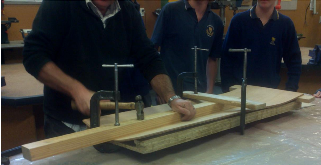
Figure 5.2 The lamination process of plywood demonstrated by the teacher to the students in the workshop.
