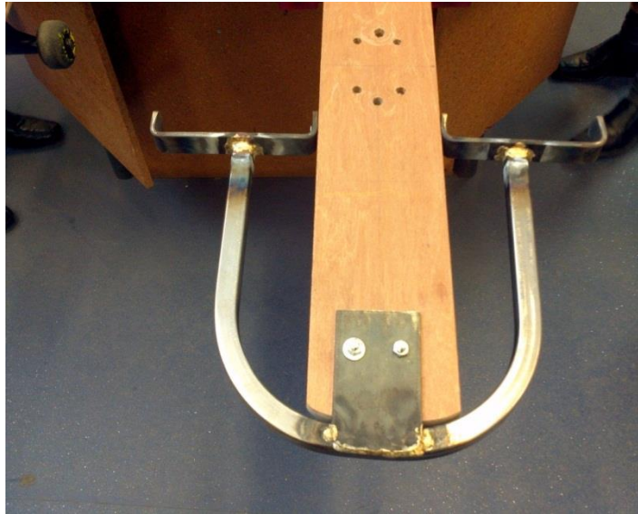
Figure 5.18 Nose cone design welded and bolted symmetrically to the frame.
