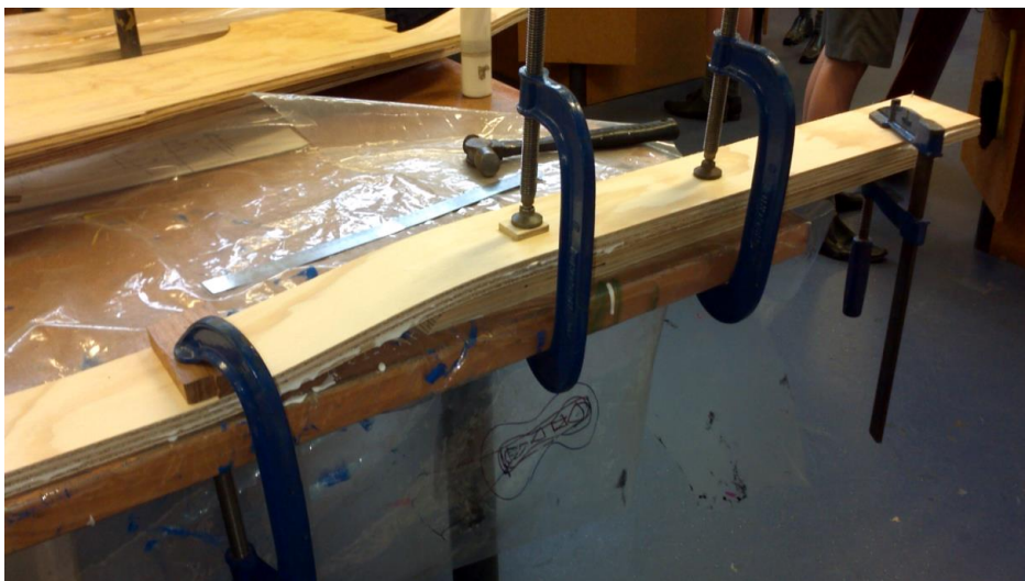
Figure 5.9 MQ's Laminated plywood for a wooden frame.
