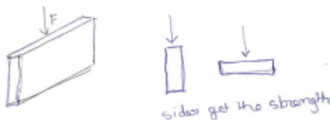
Figure 4.8 The diagram drawn by the teacher to discuss the strength of the sides of a rectangle.
