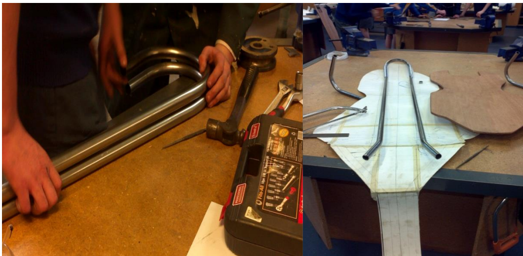
Figure 5.6 Checking symmetry and alignment with the cardboard patterns.
