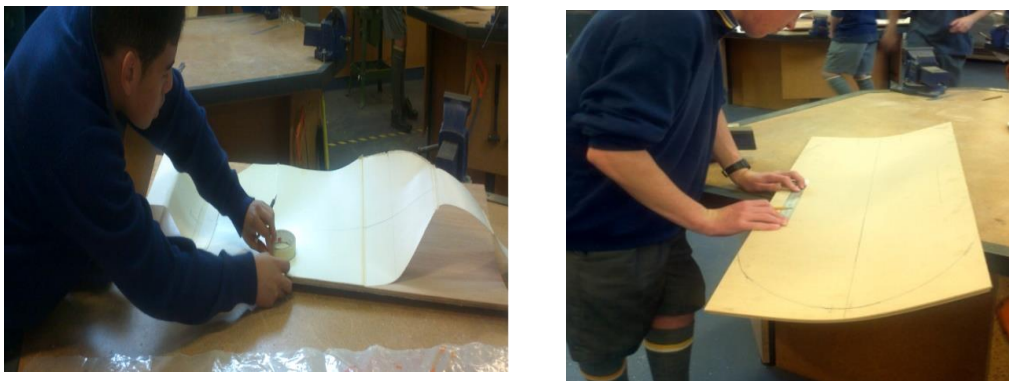
Figure 5.3 Student tracing the shape of the cardboard pattern onto the laminated plywood.
