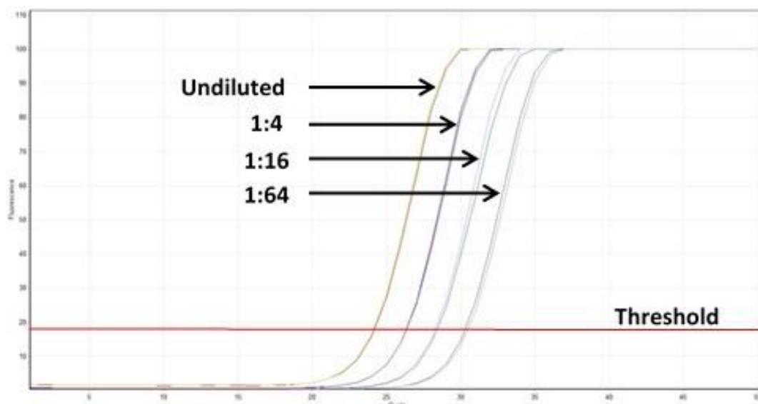
**Figure 75: Calibration curve for RT-PCR obtained from GAPDH primers. Different dilutions of template cDNA were used and the threshold was set to obtain the corresponding Ct values.**
