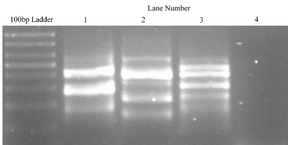
**Figure 29:** Gel image showing the first round of nested PCR. Products obtained were using the F1 and F2 primers for moronecidin and hepcidin alongside the 3' RACE outer reverse primer. The template DNA used was a combination of all *S. lalandi* tissues from which RNA was previously isolated. Lane numbering is as follows; lane 1 moronecidin F1, lane 2 moronecidin F2, lane 3 hepcidin F1, and lane 4 hepcidin F2. Refer to appendix VIII for ladder band sizing.
