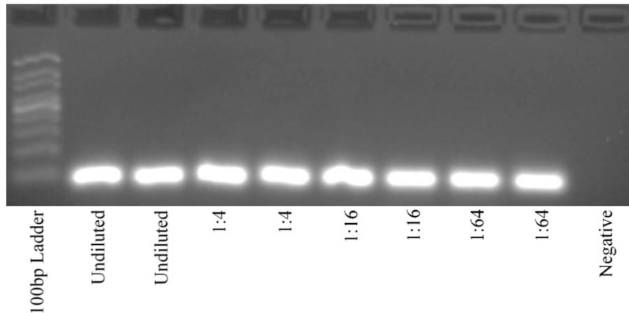
**Figure 77: Gel image showing the GAPDH RT-PCR products. Dilutions of undiluted, 1:4, 1:16 and 1:64 were performed in duplicate and run on a 1.5% agarose gel. Refer to appendix VIII for ladder band sizing**
