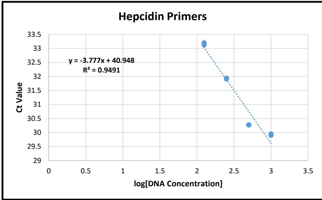
**Figure 83: Standard curve for hepcidin with Ct values plotted against the log of the template concentration. The equation of the line and the R2 value are shown.**
