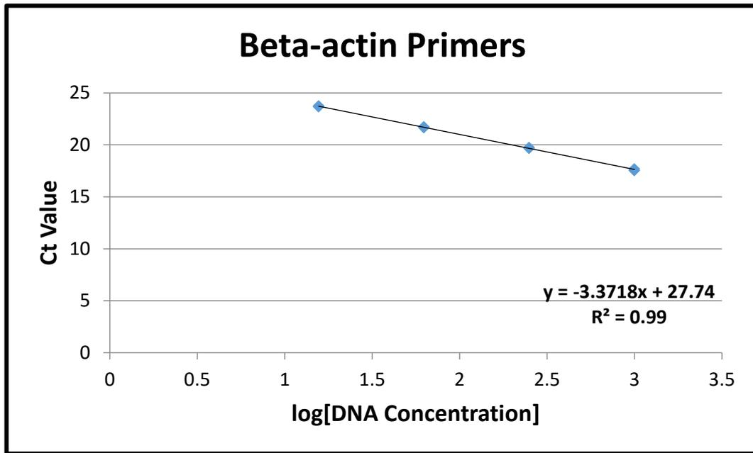
**Figure 79:** Standard curve for  $\beta$ -actin with Ct values plotted against the log of the template concentration. The equation of the line and the  $R^2$  value are shown.
