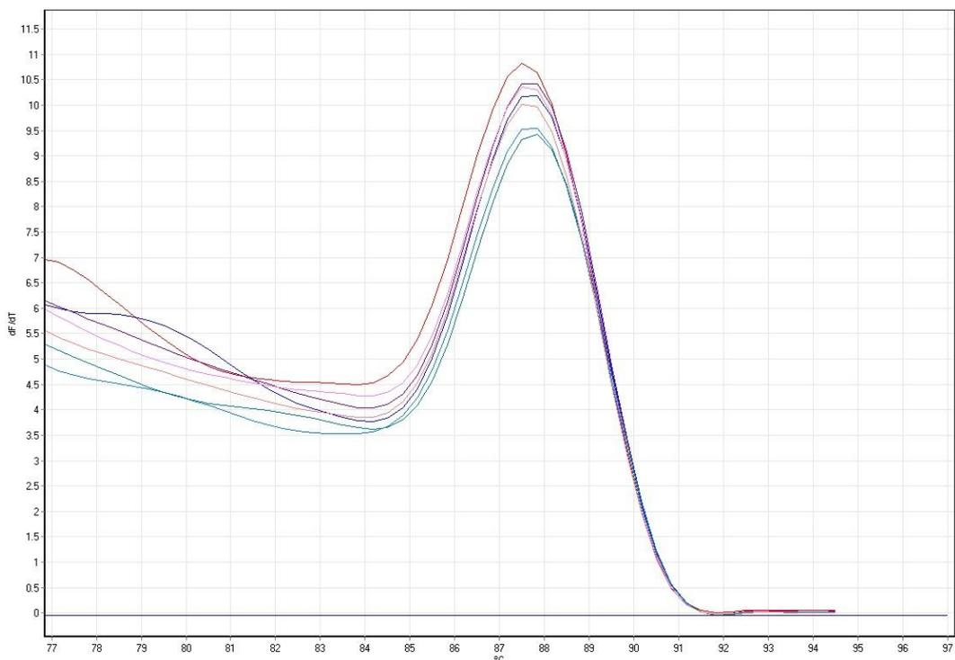
**Figure 82: The melt curve obtained using moronecidin primers. The presence of one peak showed that only one product was formed during the run.**
