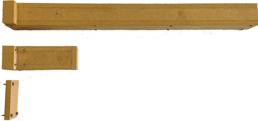
Figure 3.9: MDF acoustic loads. Top: 450 mm offset open. Middle: 150 mm offset short. Bottom: Short.
