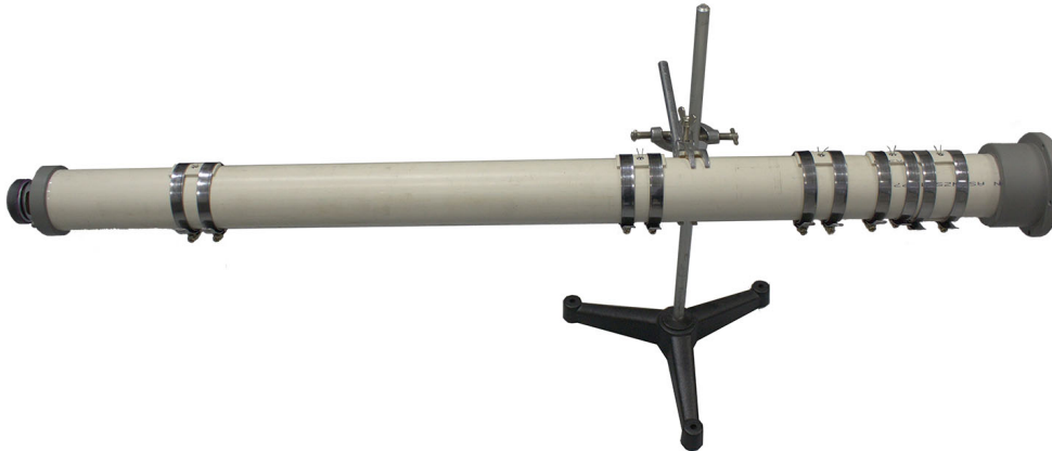
Figure 2.9: Photograph of the multi-microphone impedance tube. This revision has six microphones in five unique positions. The source is shown on the left end of the impedance tube and the coupling interface for the load on the right end.
