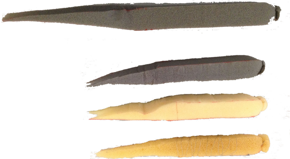
Figure 3.10: Foam wedges of different densities and lengths used as acoustic loads.
