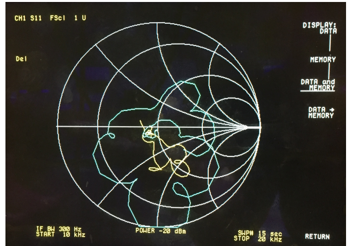
Fig. 10. Both S_{11} traces for the metal reflect and the load as displayed on the HP4395A screen. The smith chart shows amplitude information as a ratio of the source power (therefore always \leq 1 ) as the distance from the center, position indicates phase, the arcs from the outside of the circle to the far right are lines of constant phase.
