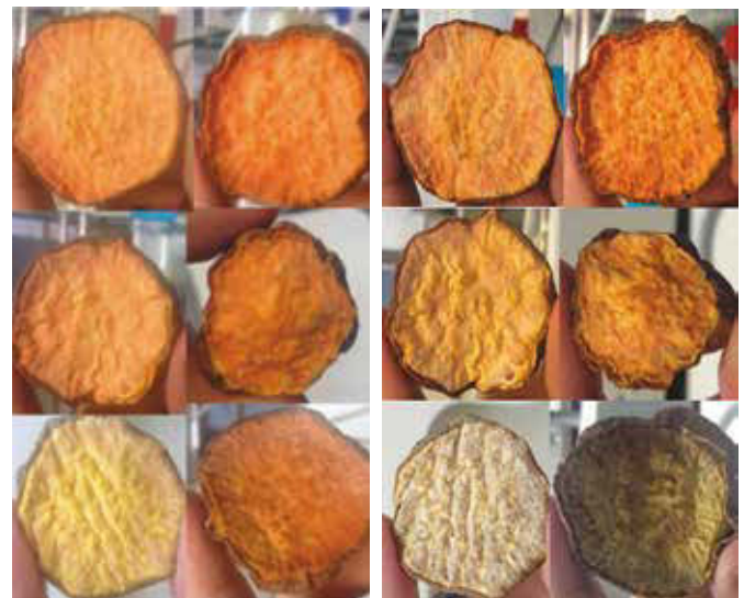
Figure 7: Appearance of kumara slices after 4 h drying at 70°C (top row), 80°C (middle row) or 90°C (bottom row). Left column has no pre-treatment; right column has 2 min microwave pre-treatment.
