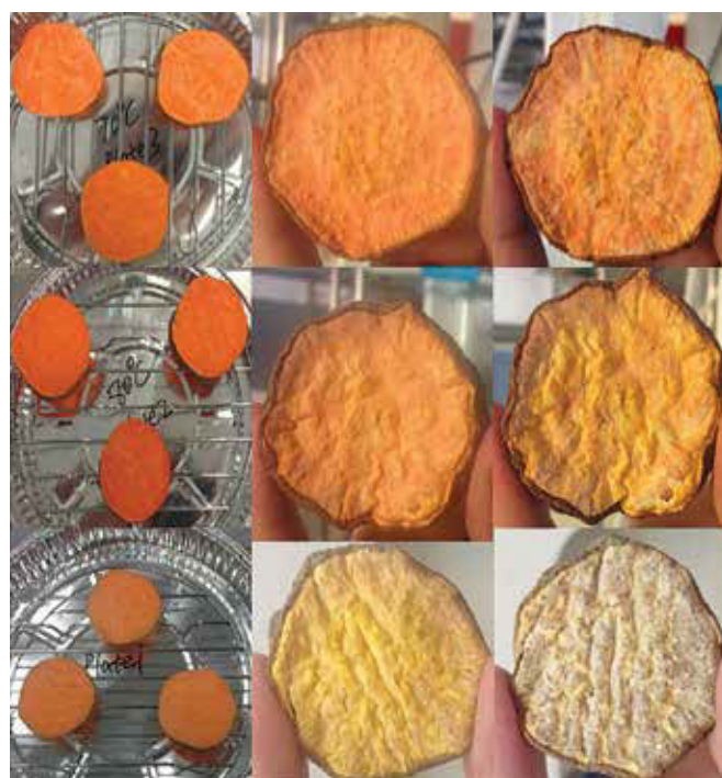
Figure 3: Orange kumara slices dried at 70°C (top row), 80°C (middle row), or 90°C (bottom row) for 0h (left column), 4h (middle column) or 10h (right column).
